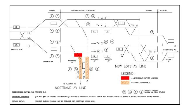
Figure 23: Alternative 6 – Track #2A Outage South of Nostrand Junction at **New Connection**
