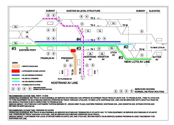
Figure 7: Alternative 4 - Track #2A / #1 Section A Outage
