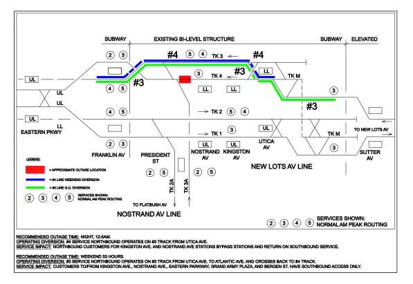
Figure 10: Alternative 4 - Track #4 Section B Outage
