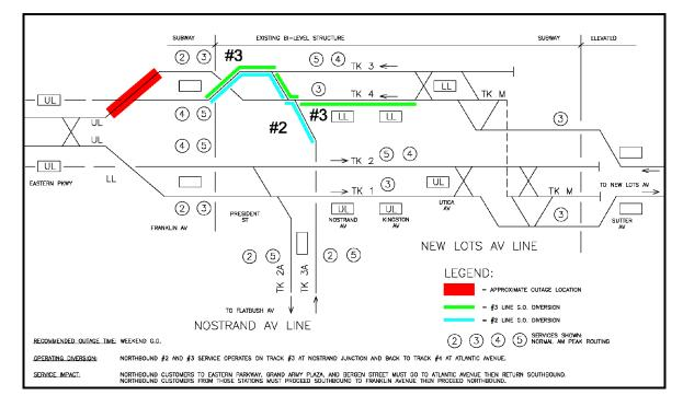
Figure 20: Alternative 6 – Track #4 Outage between Eastern Parkway and Franklin Avenue Station
