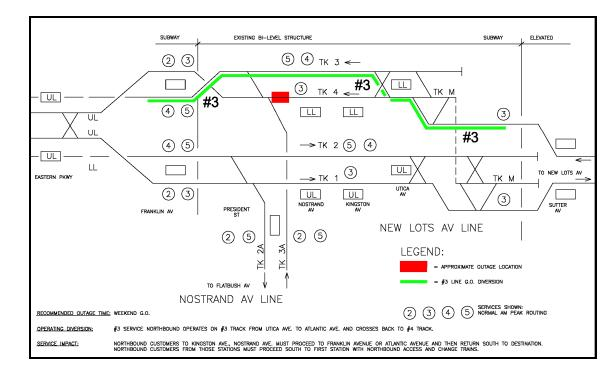
Figure 22: Alternative 6 – Track #4 Outage between Nostrand Junction and **Nostrand Avenue Station**
