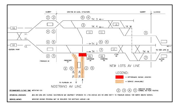
Figure 24: Alternative 6 – Track #3A Outage South of Nostrand Junction at New Connection
