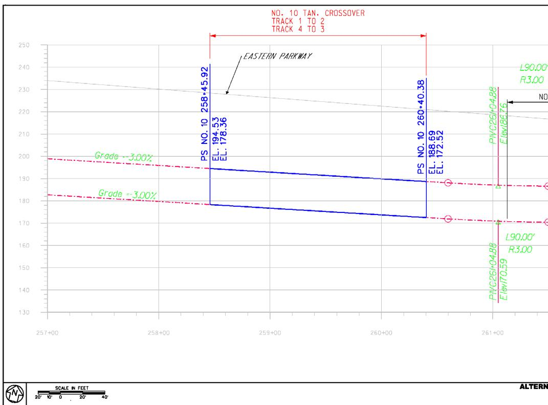
Figure 4: Alternative 4 Proposed Track Profile (Appendix H, Figure 431)
