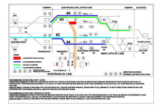
Figure 9: Alternative - Tracks #3A and #4 Section A Outage
