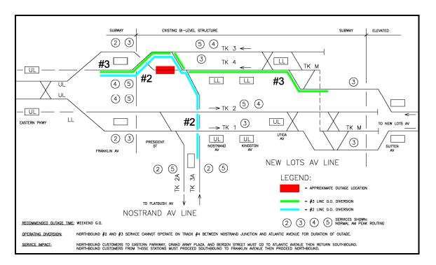
Figure 21: Alternative 6 – Track #4 Outage between Franklin Avenue Station and Nostrand Junction
