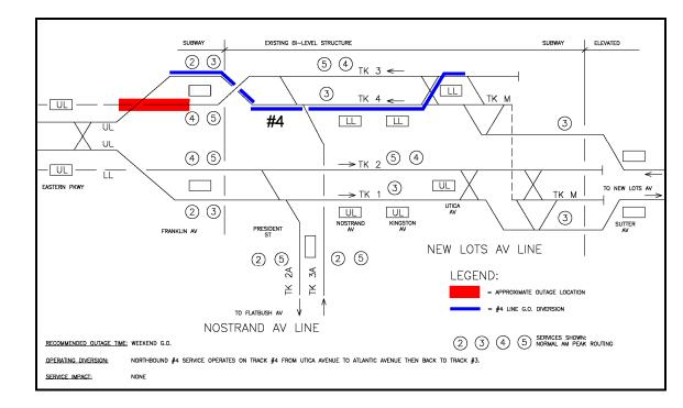
Figure 19: Alternative 6 – Track #3 Outage between Eastern Parkway and Franklin Avenue Station
