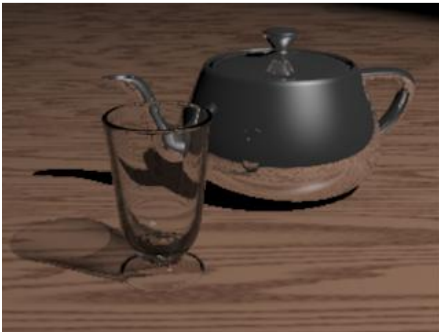
ShadingRate 1 (1 shading sample per pixel)
