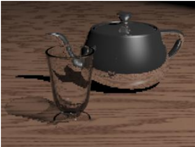
ShadingRate 4 (0.25 shading samples per pixel)
