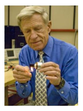
University of Utah physicist Orest Symko holds a match to a small heat engine that produces a high-pitched tone by converting heat into sound. Symko's research team is combining such heat engines with existing technology that turns sound into electricity, resulting in devices that can harness solar energy in a new way, cool computers and other electronics. Credit: University of Utah
