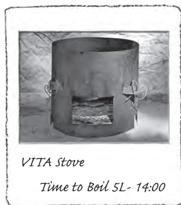
Figure 3 Fastest to Boil 5 L of Water
