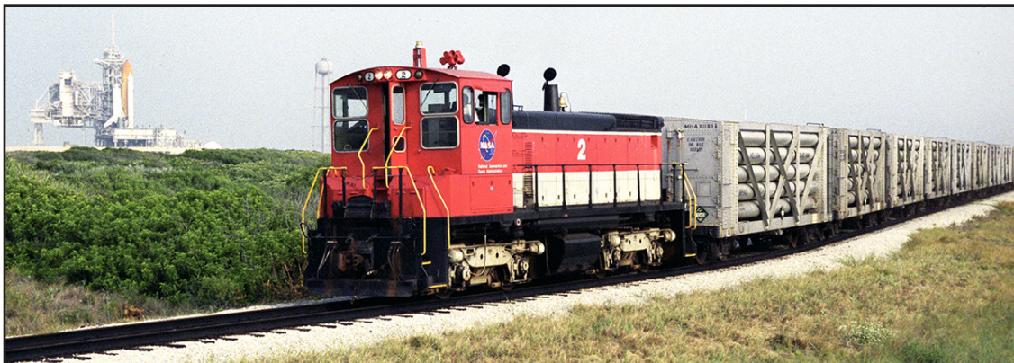
A NASA locomotive passes by a space shuttle on a launch pad at Launch Complex 39 en route to Cape Canaveral Air Force Station on the NASA Railroad. The train is delivering helium, a commodity used in launching the Titan rocket.
