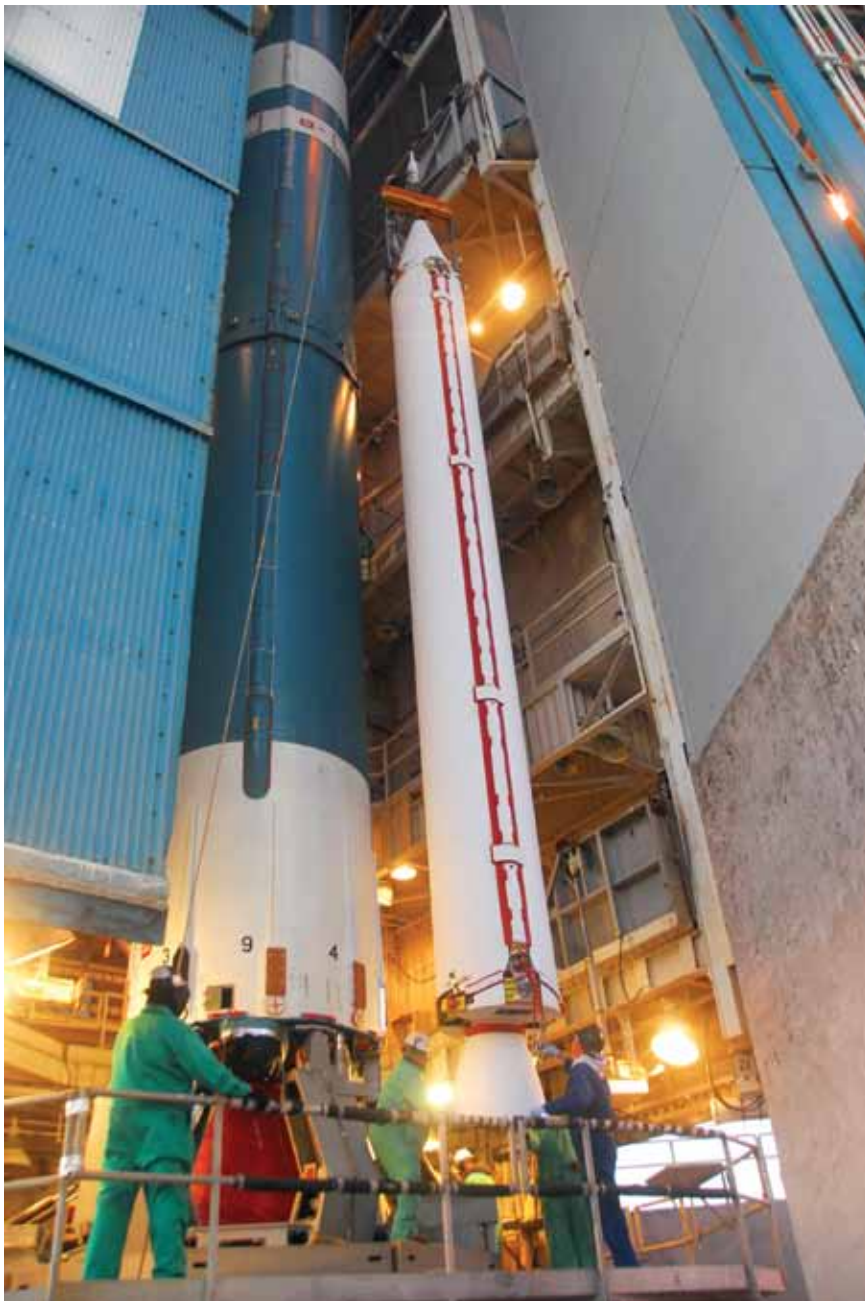
At Space Launch Complex-2 at Vandenberg Air Force Base in California, the first of three solid rocket boosters for the Delta II rocket for launch of NASA's Wide-field Infrared Survey Explorer (WISE) is positioned next to the rocket's first stage in the pad's mobile service tower, Oct. 21, 2009.
