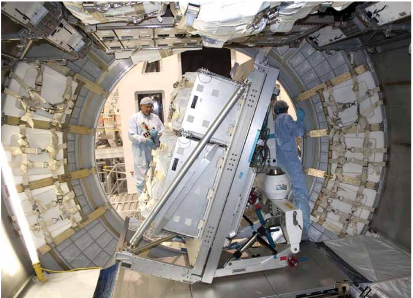
In Kennedy Space Center's Space Station Processing Facility, May 11, 2010, technicians disconnect the remaining racks from the inner walls of multi-purpose logistics module Leonardo after its return from the STS-131 mission to the International Space Station.
