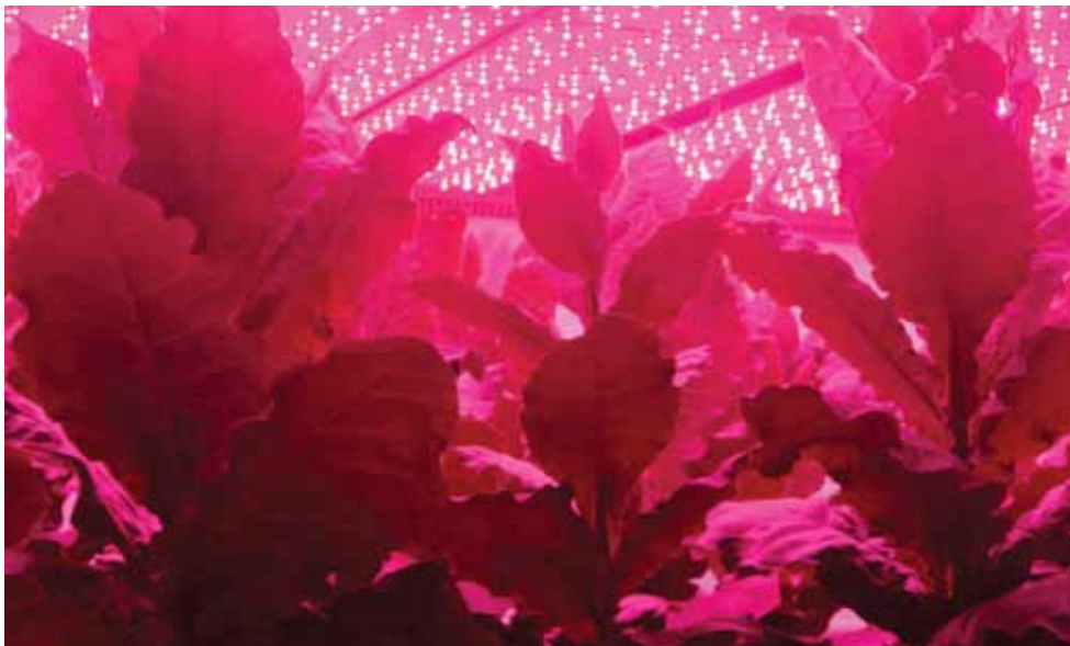
New light-emitting diode (LED) arrays for collapsible plant growth chambers were the focus of research at Kennedy Space Center's Space Life Sciences Laboratory.
