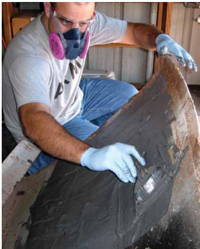
A technician at Kennedy Space Center applies the Activated Metal Treatment System to a piece of painted metal beam. The technology that breaks down PCBs in paints was developed by researchers at Kennedy and the University of Central Florida.
