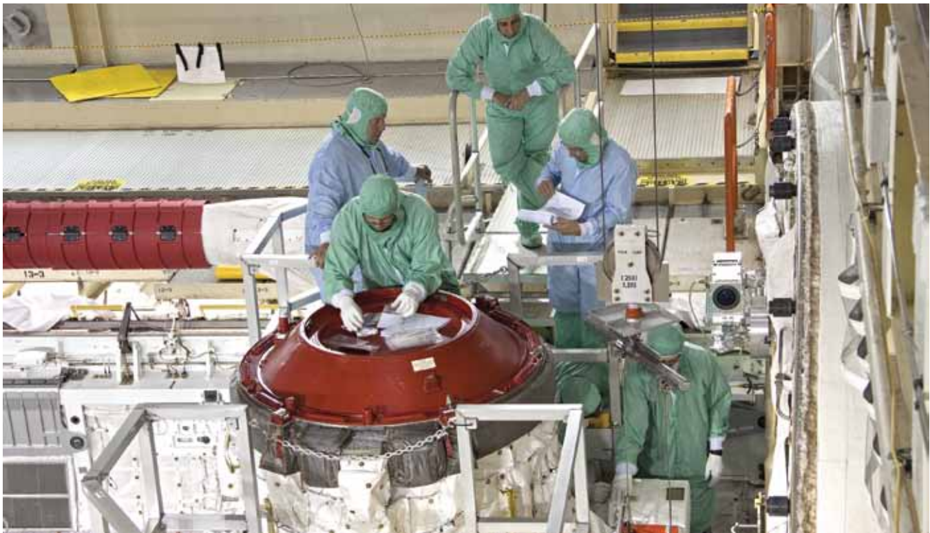
Inside Kennedy Space Center's Orbiter Processing Facility-3, technicians install a DragonEye proximity sensor, developed by SpaceX, in space shuttle Discovery on July 28, 2010. DragonEye is a laser imaging detection and ranging sensor that was tested on Discovery's docking operations with the International Space Station during the STS-133 mission.
