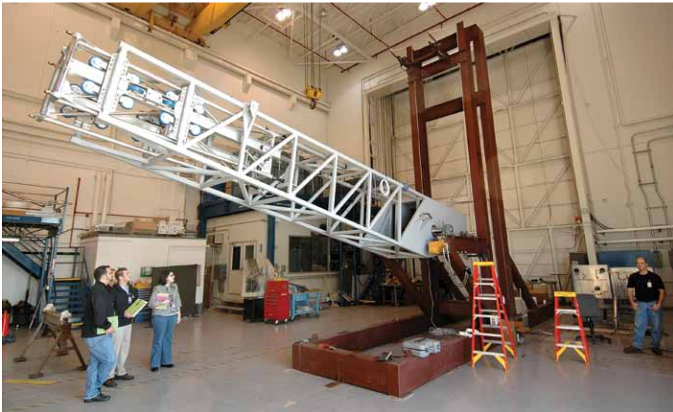
Engineers check the mobility of the new Tilt-Up Umbilical Arm (TUUA) at Kennedy Space Center's Launch Equipment Test Facility on Oct. 21, 2010.
