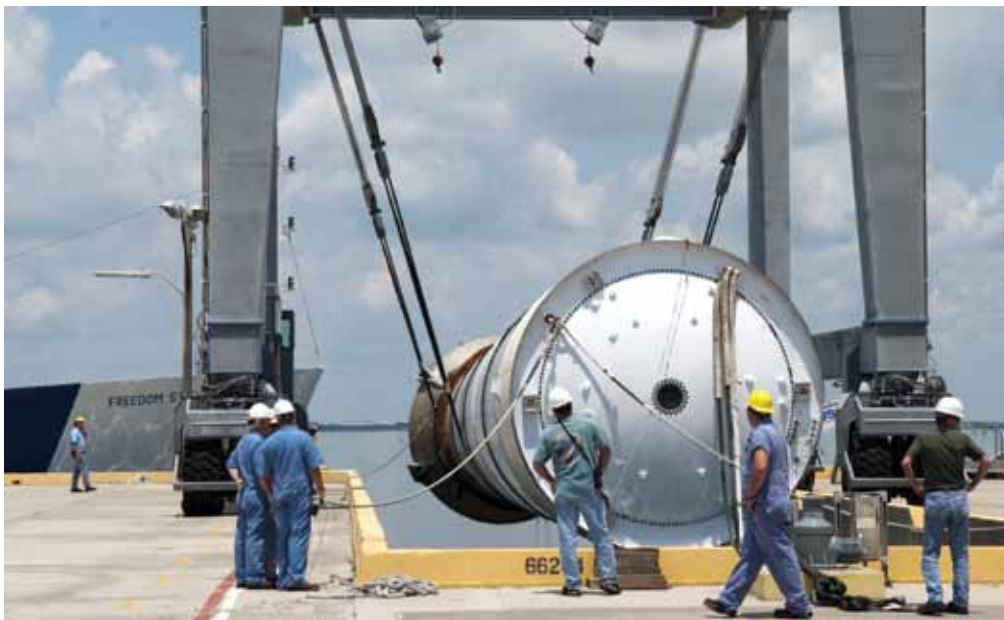
A mobile gantry crane lifts one of the solid rocket boosters used during space shuttle Atlantis' STS-132 launch in May 2010 from a hoisting slip at the Solid Rocket Booster Disassembly Facility at Hangar AF on Cape Canaveral Air Force Station in Florida.
