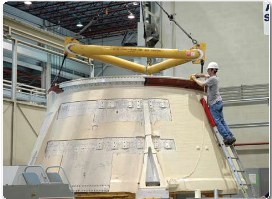
Below: In the Assembly and Refurbishment Facility at Kennedy Space Center, a worker attaches an overhead crane to the aft skirt for the Ares I-X flight test. The segment is being lifted into a machine shop work stand for drilling modifications.
