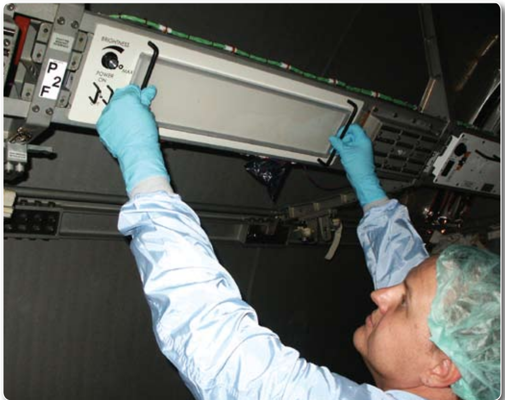
Bionetics Corp. Lead Mechanical Engineer Todd Mortenson performs a fit check of the Solid State Lighting Module, or LED light, in a lighting fixture slot of a multi-purpose logistics module in the Space Station Processing Facility at Kennedy Space Center.
