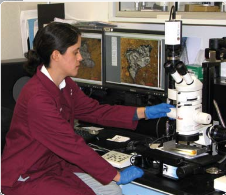
Clara Wright, a Kennedy Space Center materials engineer, uses a stereomicroscope to analyze small fragments of the International Space Station's damaged starboard Solar Alpha Rotary Joint returned on mission STS-120.
