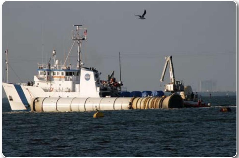
Above: The Freedom Star, one of NASA's solid rocket booster retrieval ships, tows a solid rocket booster to Hangar AF at Cape Canaveral Air Force Station. The booster is from the STS-123 mission, which launched Endeavour on March 11, 2008.
