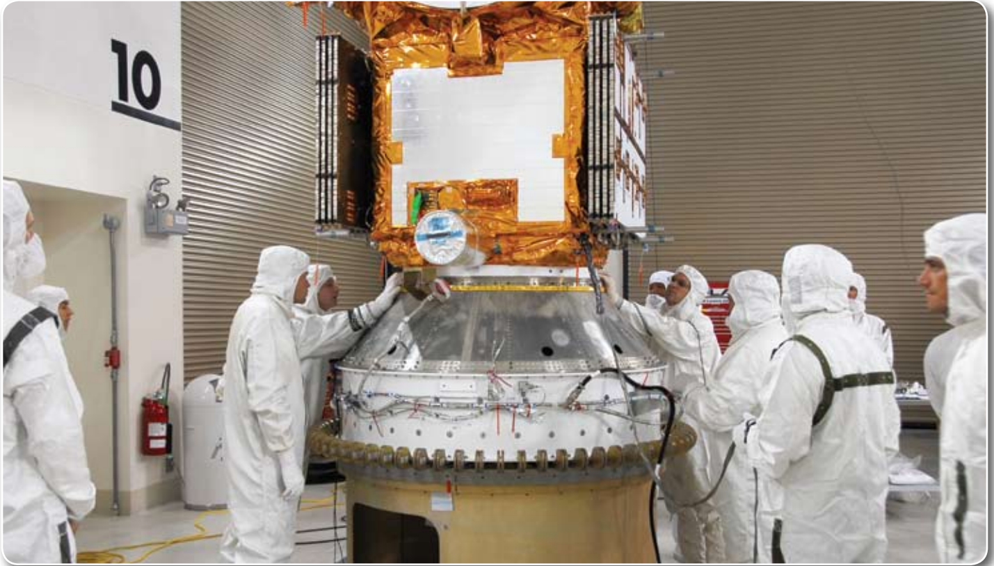
At Vandenberg Air Force Base in California, engineers checked the fit of the Ocean Surface Topography Mission, or OSTM/Jason-2 spacecraft as it was lowered onto the payload attach fitting for installation. The payload attach fitting is the interface with the Delta II launch vehicle. OSTM/Jason-2 launched aboard a Delta II on June 20, 2008, at 12:46 a.m. PDT.
