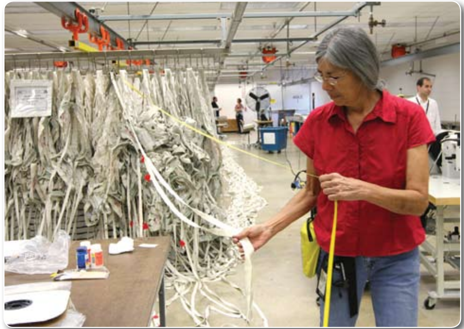
Above: Inside the Parachute Refurbishment Facility at Kennedy Space Center, Deborah Coombs, senior parachute technician, measures suspension lines for the Ares I main canopy. Ares I is an in-line, two-stage rocket that will transport the Orion crew exploration vehicle to low Earth orbit.
