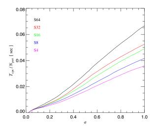
**Figure 21.** Total elapsed wall-clock time per particle of each test run as a function of cosmological scalefactor. The elapsed run times of each simulation have been multiplied by the processor number, and normalized by the particle number.
