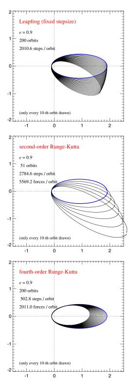
**Figure 4.** A Kepler problem of high eccentricity evolved with different simple time integration schemes, using an equal time-step in all cases. Even though the leapfrog and the second-order Runge–Kutta produce comparable errors in a single step, the long-term stability of the integration is very different. Even a computationally much more expensive fourth-order Runge–Kutta scheme, with a smaller error per step, performs dramatically worse than the leapfrog in this problem.
