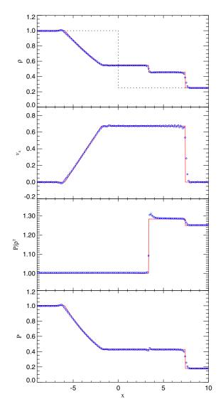
**Figure 9.** Sod shock test carried out in three dimensions. The gas is initially at rest with  $\rho_1 = 1.0$ ,  $P_1 = 1.0$  for x < 0, and  $\rho_2 = 0.25$ ,  $P_2 = 0.1795$  for x > 0. The numerical result is shown with circles (with a spacing equal to the mean particle spacing in the low-density region) and compared with the analytical result at t = 5.0. A shock of Mach number M = 1.48 develops.
