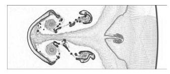
**Figure 17.** Local gradients in the gas density field at time t = 4.5, visualized by a grey-scale image with intensity proportional to log ( $|\nabla \rho|/\rho$ ). Clearly visible are the two pairs of primary and secondary vortices, as well as the stem of the backflow. The region shown has a size of  $31.25 \times 12.5$ .
