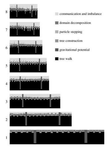
**Figure 18.** Diagram for the time consumption of a rather small galaxy collision simulation evolved with a different number of processors between one and eight. We show a sample of 64 time-steps in each case, each represented by a vertical bar with a width proportional to the elapsed wall-clock time during this step. Each step is additionally subdivided into different constituent parts, drawn in different shades of grey as indicated in the legend.
