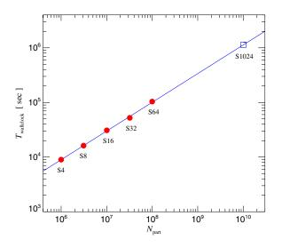
**Figure 20.** Wall-clock times consumed by the test runs of the simulation series. An extrapolation to the size of a  $2160^3$  simulation suggests that it should require about  $1.1 \times 10^6$  s on 1024 processors.
