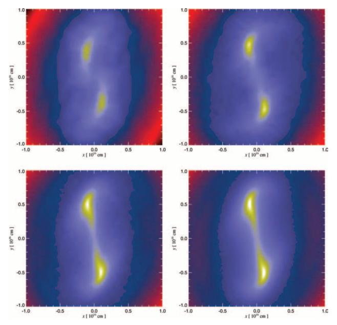
**Figure 11.** Resolution study for the 'standard isothermal collapse' simulation. We show the gas density in a slice trough the centre of the simulated volume at 1.24 free-fall times, roughly when the two perturbations at the ends of the bar-like structure become self-gravitating and undergo gravitational collapse. From the top left to the bottom row, the particle number increases from  $3.3 \times 10^4$  to  $1.71 \times 10^7$  by factors of 8.
