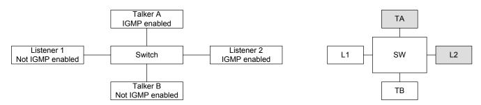
Figure 3 – IGMP registration with dumb switch
