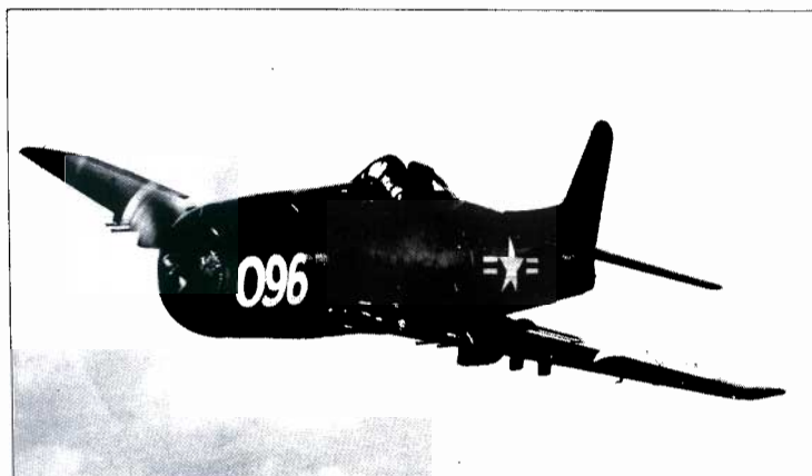
Photographed while on manufacturer's test flying prior to US Navy acceptance, this is a cannon-armed F8F-1B, BuAer no. 122096. The larger guns much more than doubled the firepower and had little effect on any aspect of performance except rate of climb. Many F8Fs, including 122096, had two dorsal whip radio aeriels.
