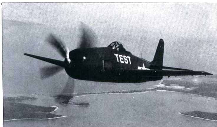
The very first Bearcat was BuAer no. 90460, seen here over the Long Island shore in the hands of company pilot Bob Hall. Compared with every other F8F this XF8F-1 was shorter in span but longer in the body, and it also lacked a dorsal fin. It was current practice to write TEST as a warning to other air traffic nearby.
