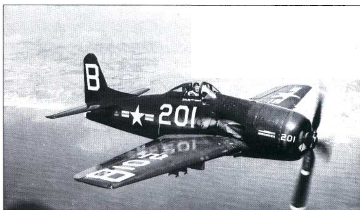
This standard F8F-1, BuAer no. 95318, is seen flying with a post-war US Navy fighter squadron. Note the underwing pylons for two tanks or bombs and four HVARs (high-velocity aircraft rockets) and the scorching of fuselage paint downstream of the grouped exhaust outlet.
