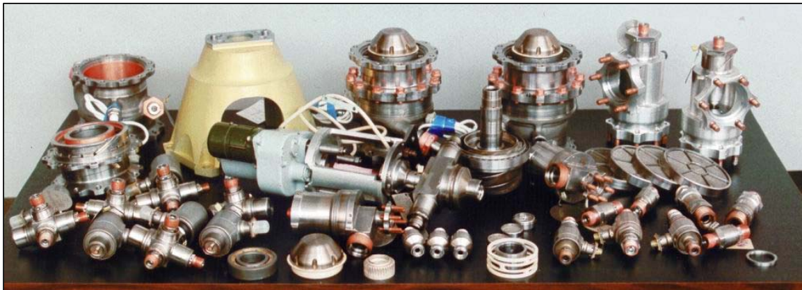
Main oxygen pump parts, manufactured by powder technology (HIP) method
