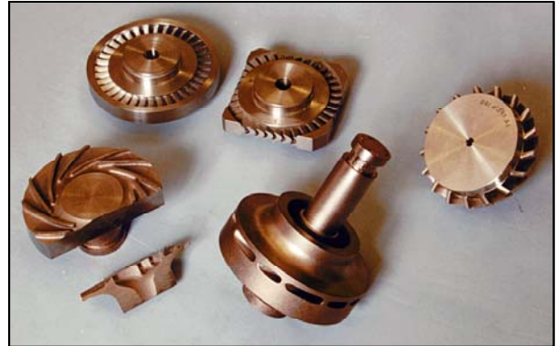
Main oxygen pump parts, manufactured by powder technology (HIP) method
