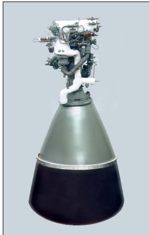
RD0146 engine I_{sp.} = 463 \text{ kgf}\cdot\text{s}/\text{kg}
