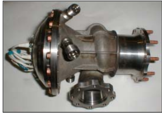
Hydrogen boost pump
