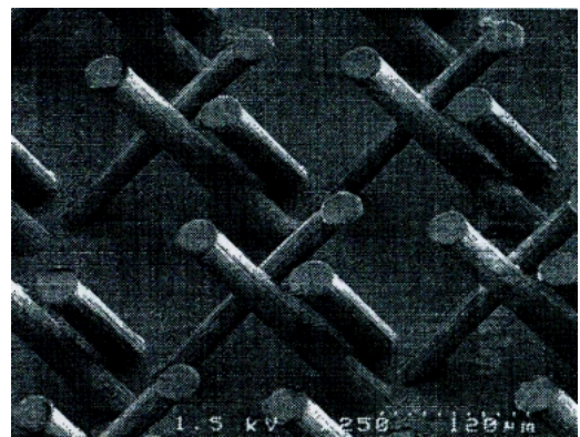
Fig. 11 Example of 3D microstructure fabricated by multi-step x-ray exposure 45) .
