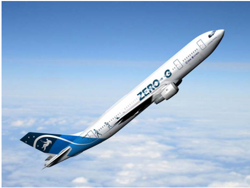
Fig. 7: Airbus A300 'Zero-G' aircraft, operated by Novespace, used by ESA for its Microgravity Research Campaigns (credit: Novespace)
