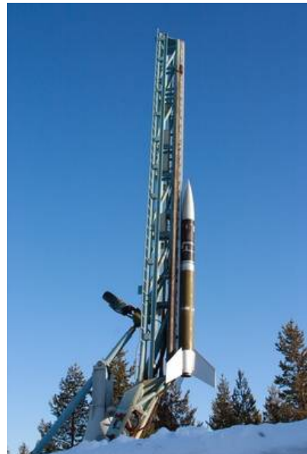
Fig. 6: Used in the REXUS programme, the Improved Orion M112 is an unguided solid-propellant single-stage rocket, launched from Kiruna in Sweden (SNSB)
