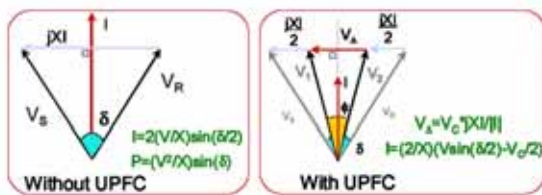
Figure 11. UPFC operation
