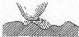
Fig. 4. An enlarged section of an arc, and it is suggested that the action of a crystal detector is due to an electron discharge, in some respects having similar properties.
