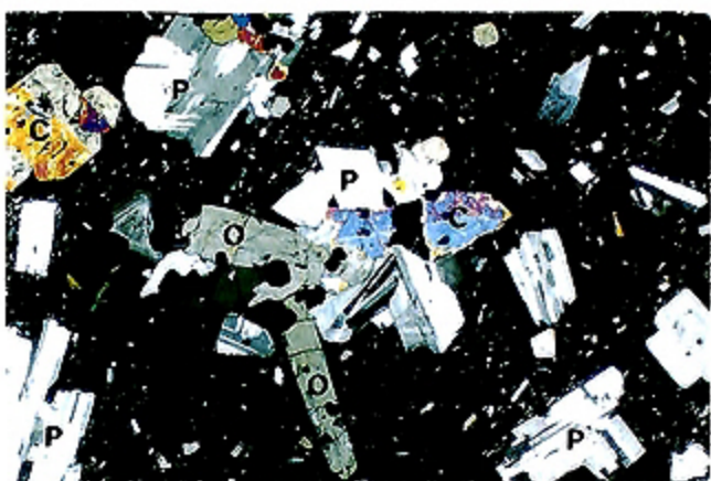
写真 6 金曜海山北東峰産の玄武岩質安山岩 (940418 site3-1, クロスニコル, 幅 5mm, P: 斜長石, C: 単斜輝石, O: 斜方輝石) Photo 6 Basaltic andesite from the North-East Top of Kinyo Seamount. (940418 site3-1, Crossed nicols, Width of field of view is 5mm, P: plagioclase, C: clinopyroxene, O: orthopyroxene)
