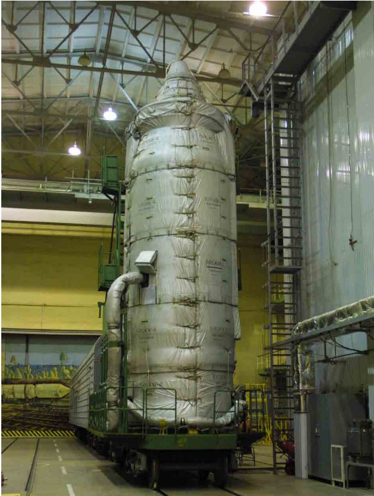
Figure 1-26 Rockot upper composite with thermal conditioning unit rail car protected by thermal cover for transfer to the launch pad.
