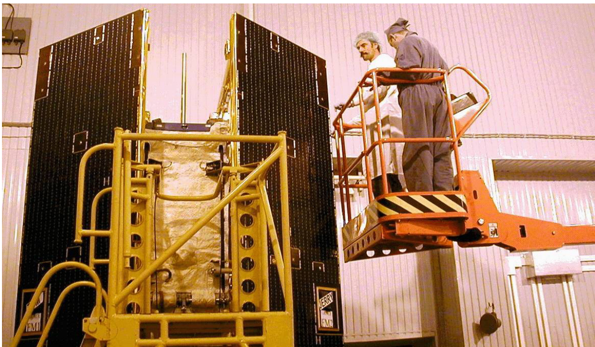
Figure 1-16 Spacecraft installation on the multi-satellite dispenser (GRACE, 2002).
