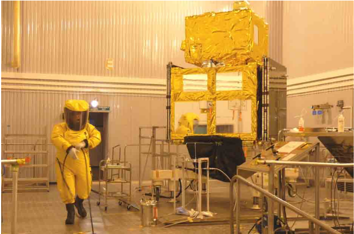
Figure 1-18 Spacecraft hydrazine fuelling on EUROCKOT fuelling platform.
