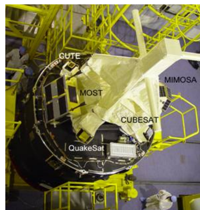
Figure 4-2 Integrated MOM payload with main payload simulator.
