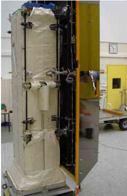
Figure 4-15 Example of side-mounted multiple satellite dispenser system for two spacecraft (GRACE), only one spacecraft attached.
