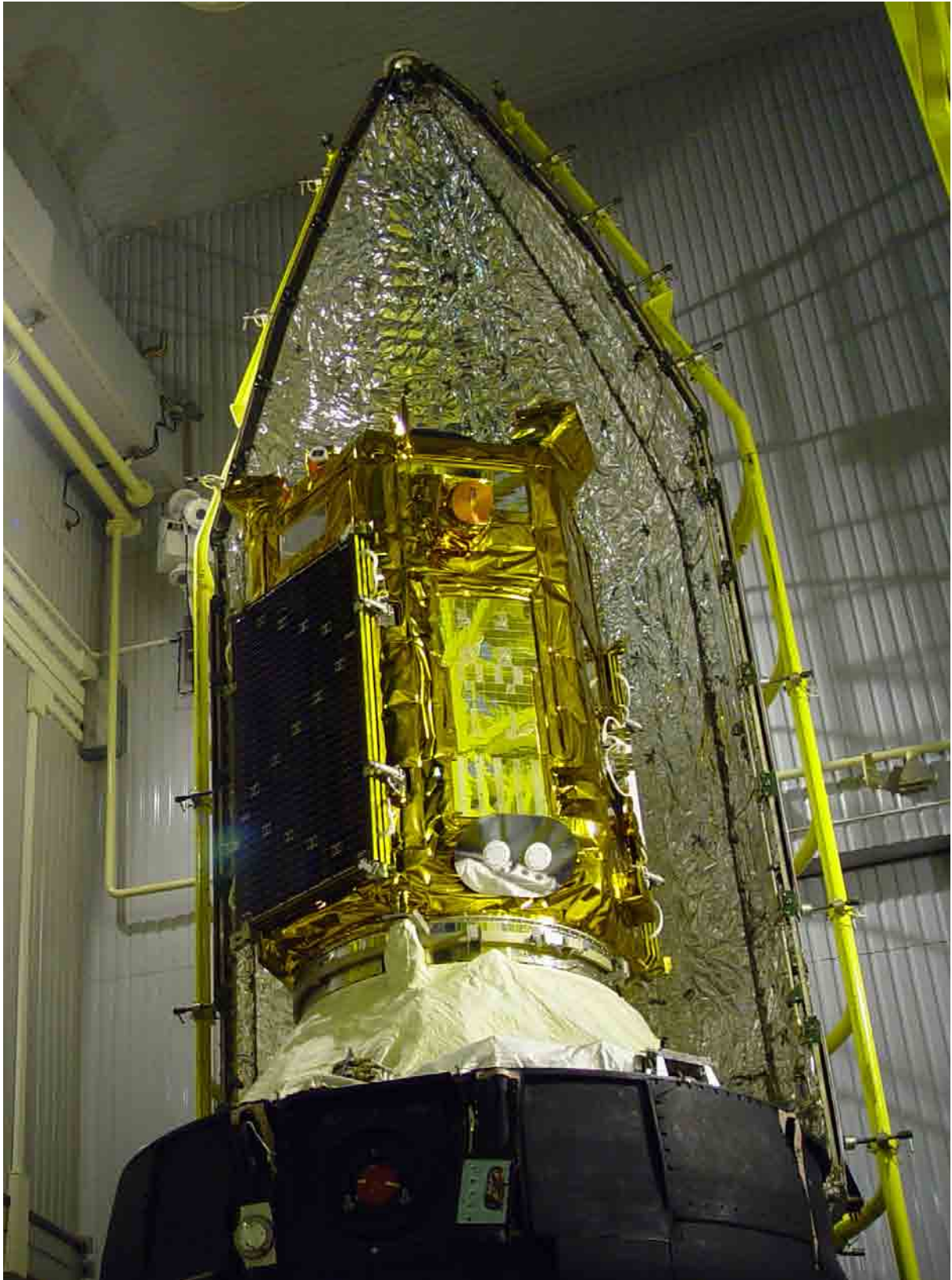
Figure 1-24 Final encapsulation operations (SERVIS-1, 2003).
