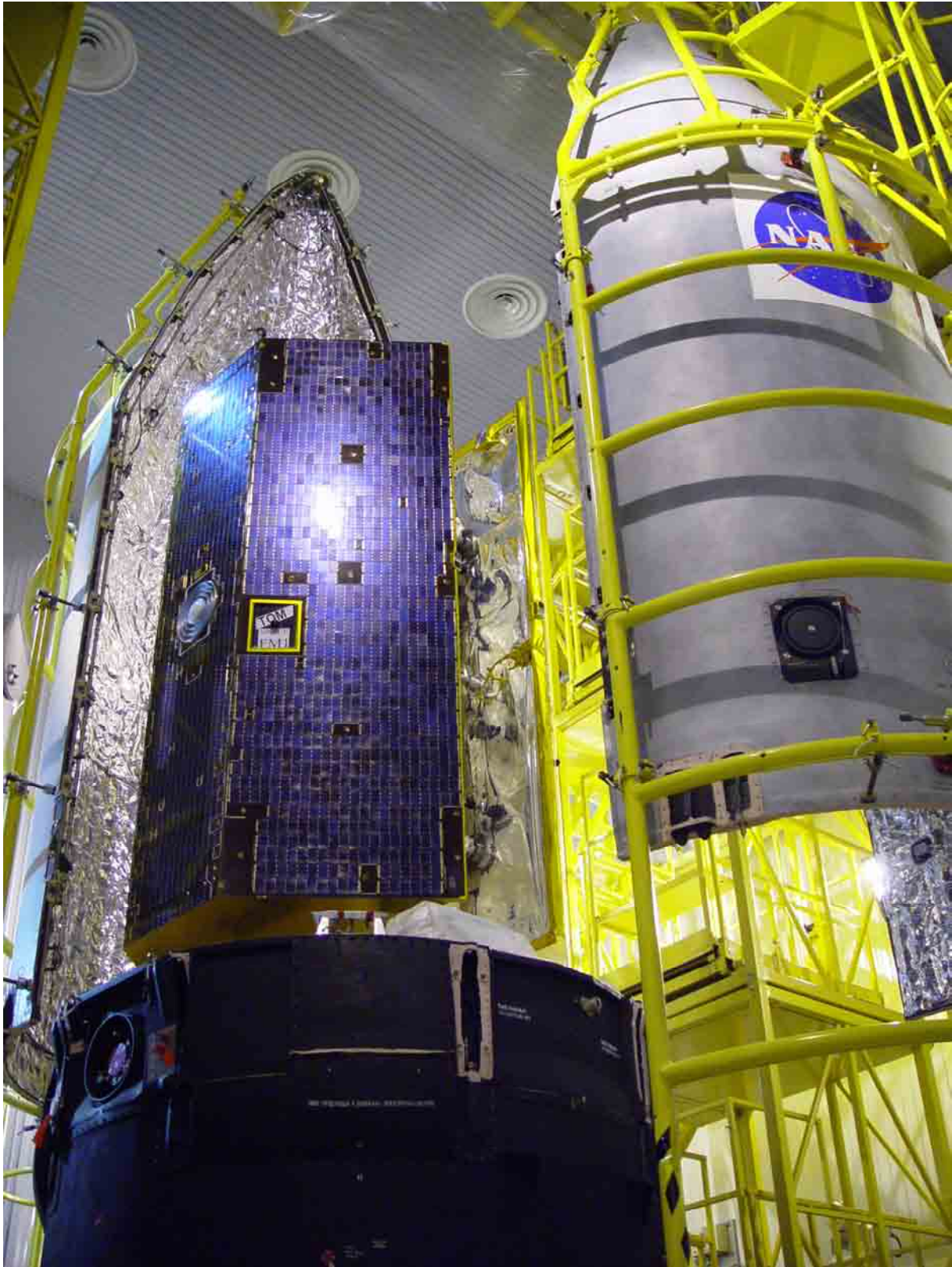
Figure 1-23 Final encapsulation operations (GRACE, 2002).
