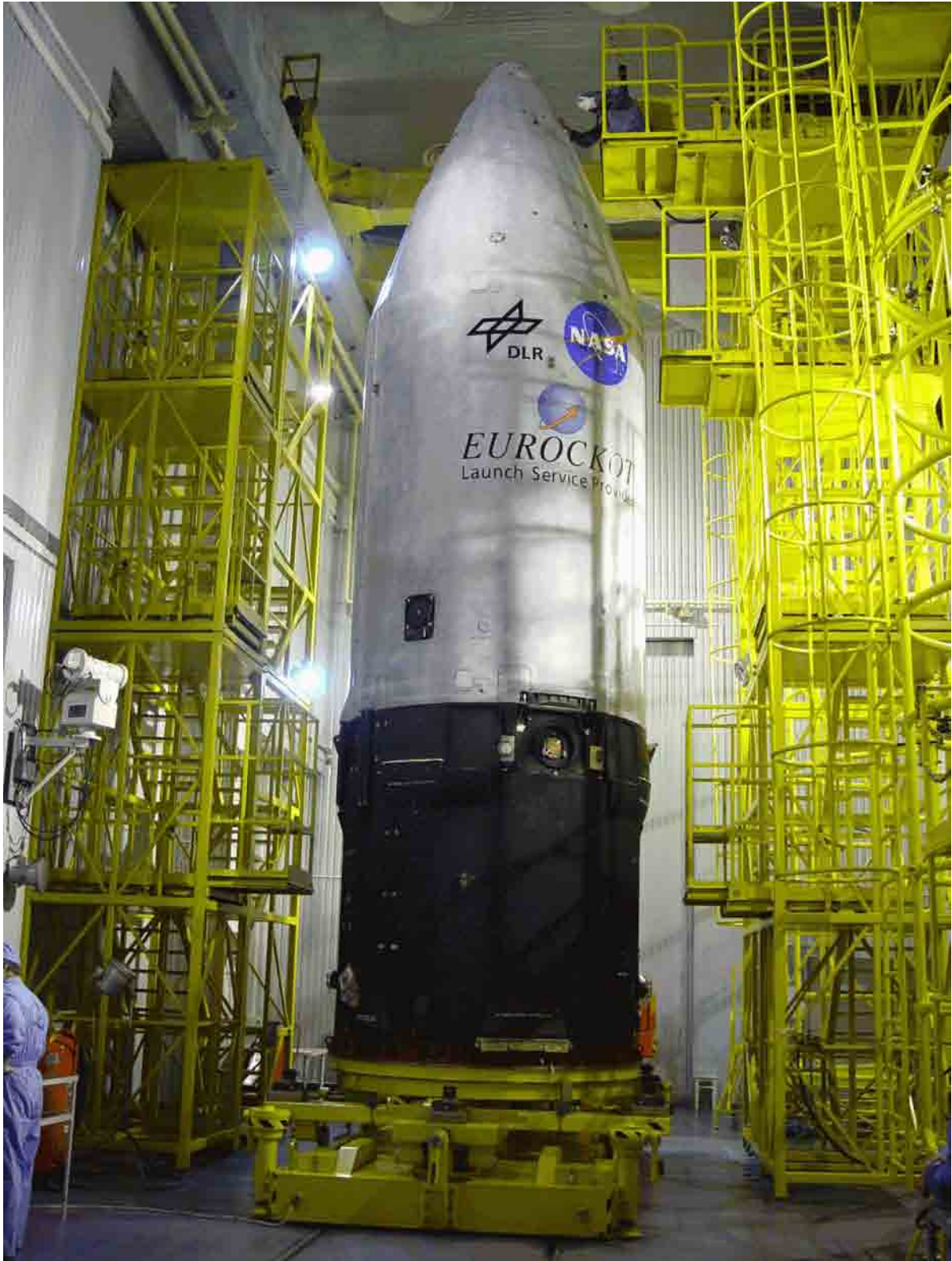
Figure 1-25 Completion of payload encapsulation (GRACE, 2002).
