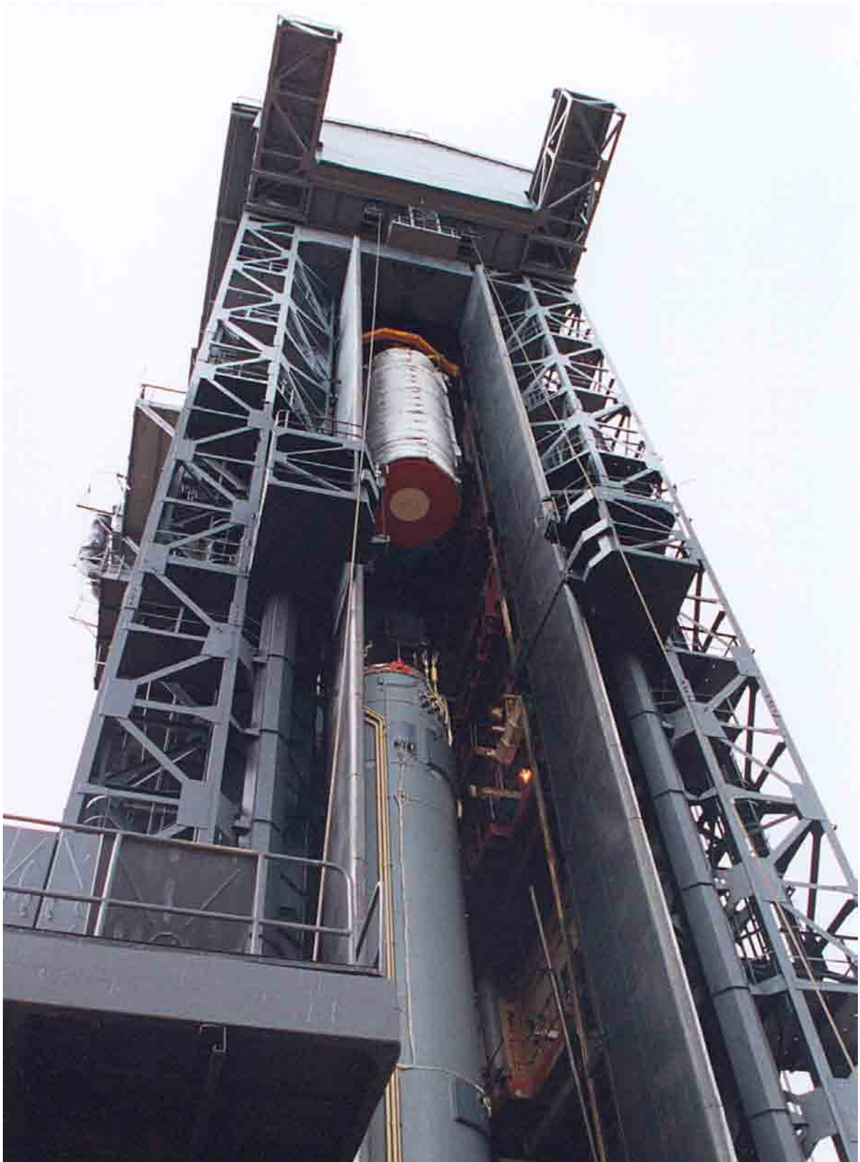
Figure 1-29 Stacking of upper composite onto the Rockot booster.
