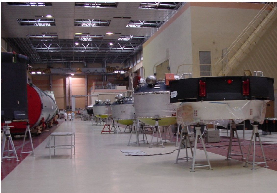
Figure 1-38 Breeze-KM upper stage production at KSRC, Moscow.
