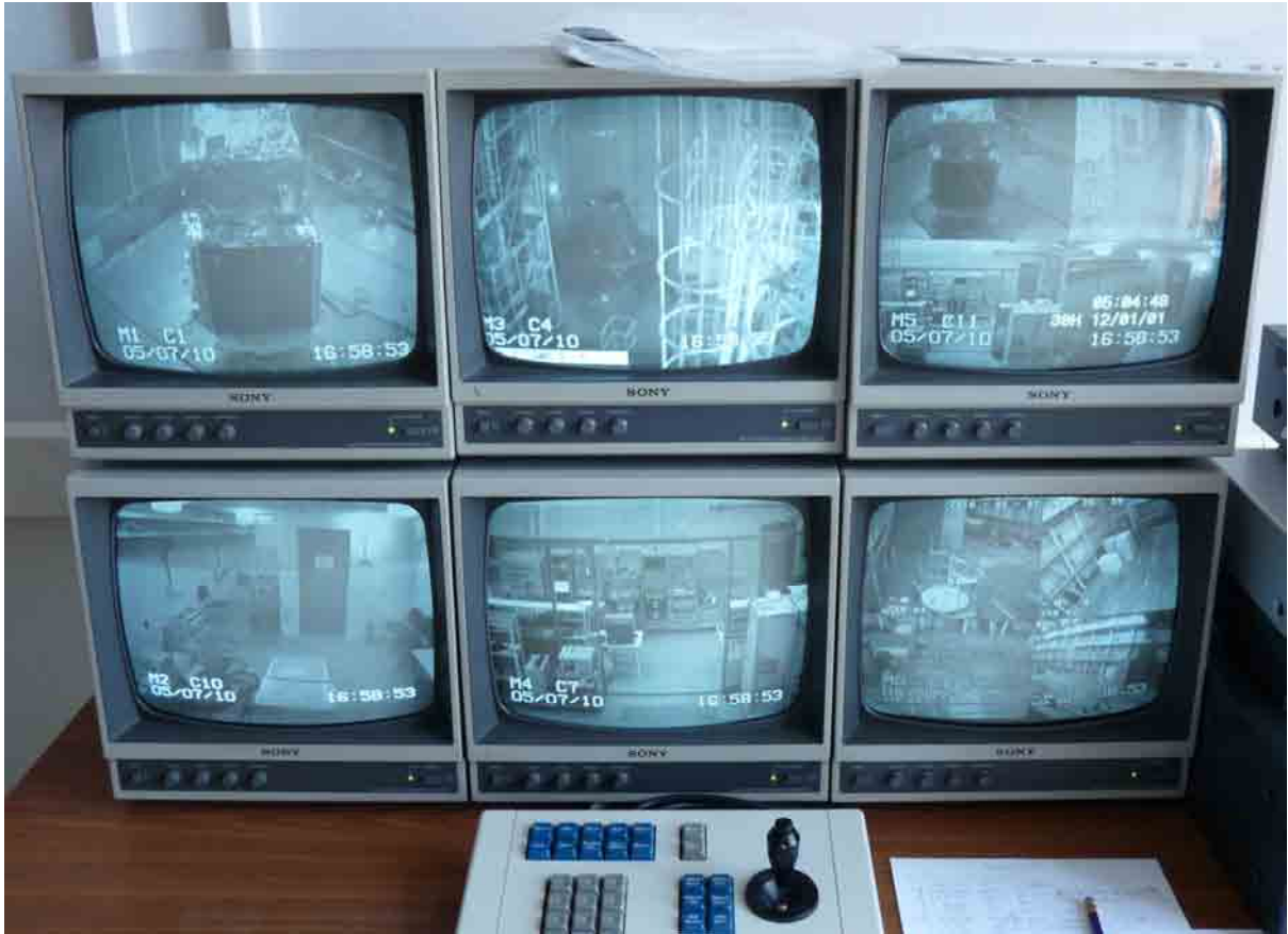
Figure 1-17 Controls of EUROCKOT Closed Circuit Television (CCTV) system for Customer usage.
