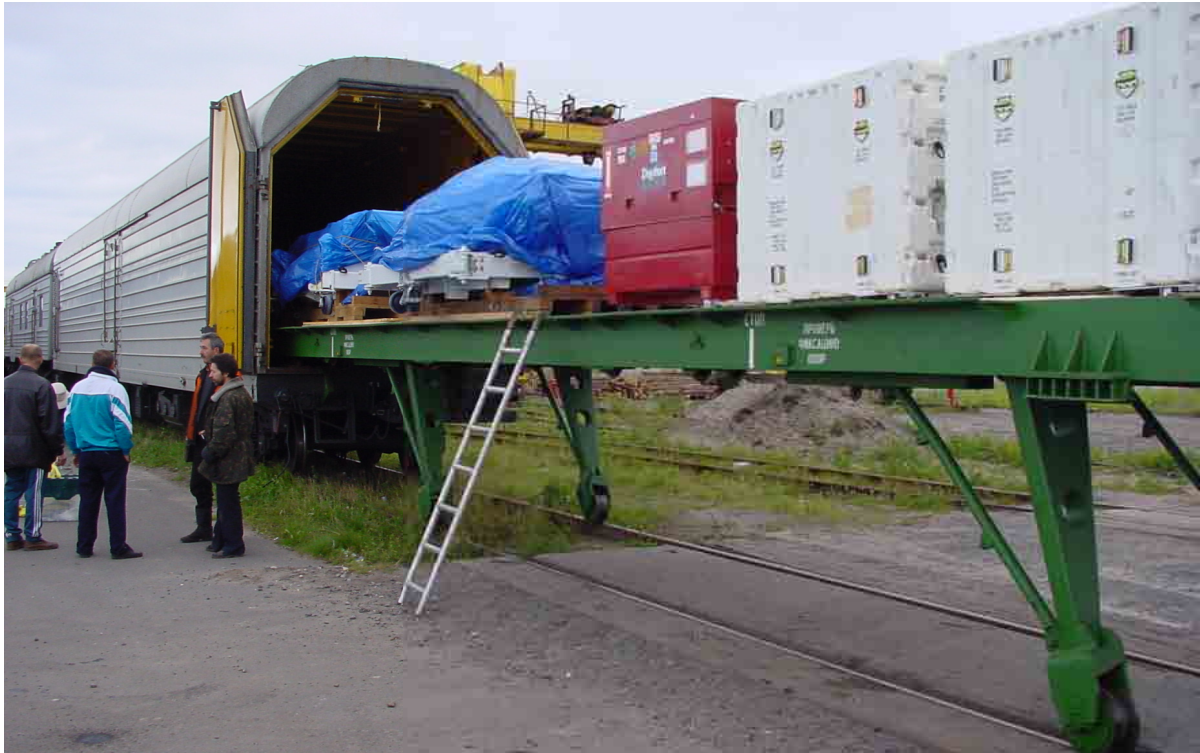
Figure 1-7 Thermally controlled railroad car for transportation of specific GSE.
