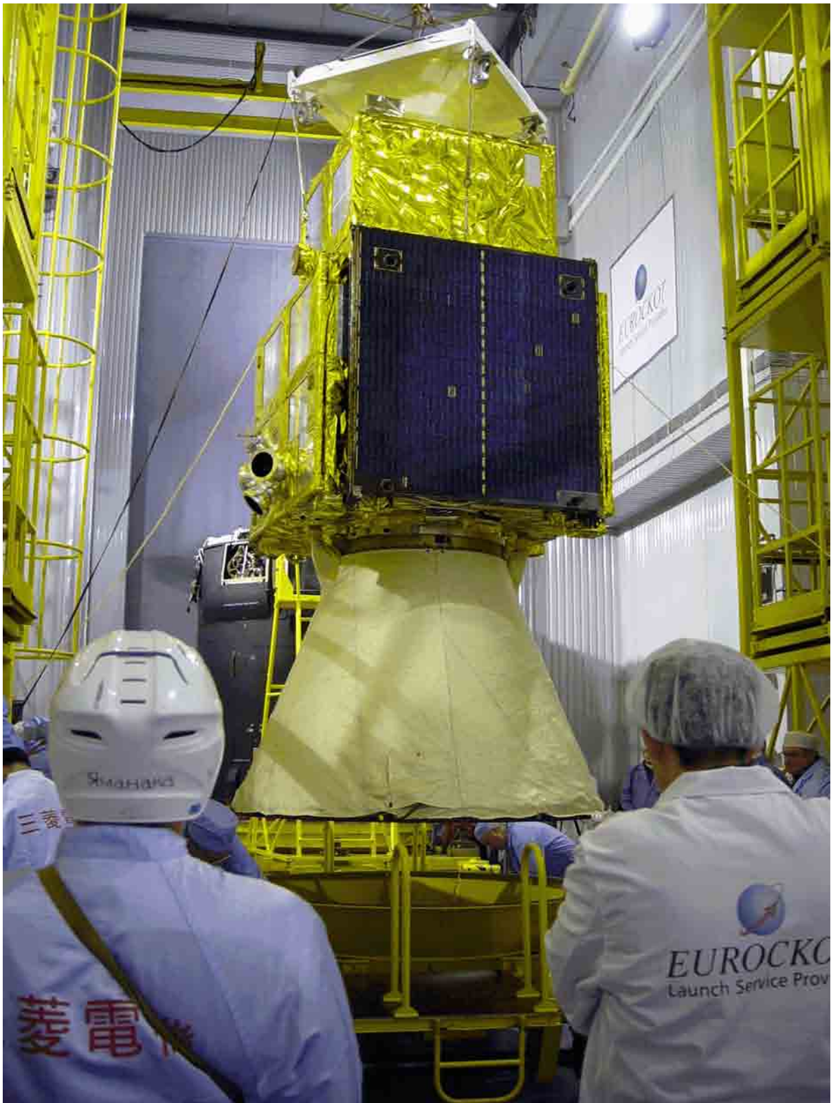
Figure 1-20 Transfer of integrated spacecraft and adapter for mating operations with the Breeze-KM upper stage (SERVIS-1, 2003).
