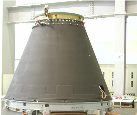
Figure 4-12 Elongated conical payload adapter for the CASA CRSS 937 SRF clamp band.
