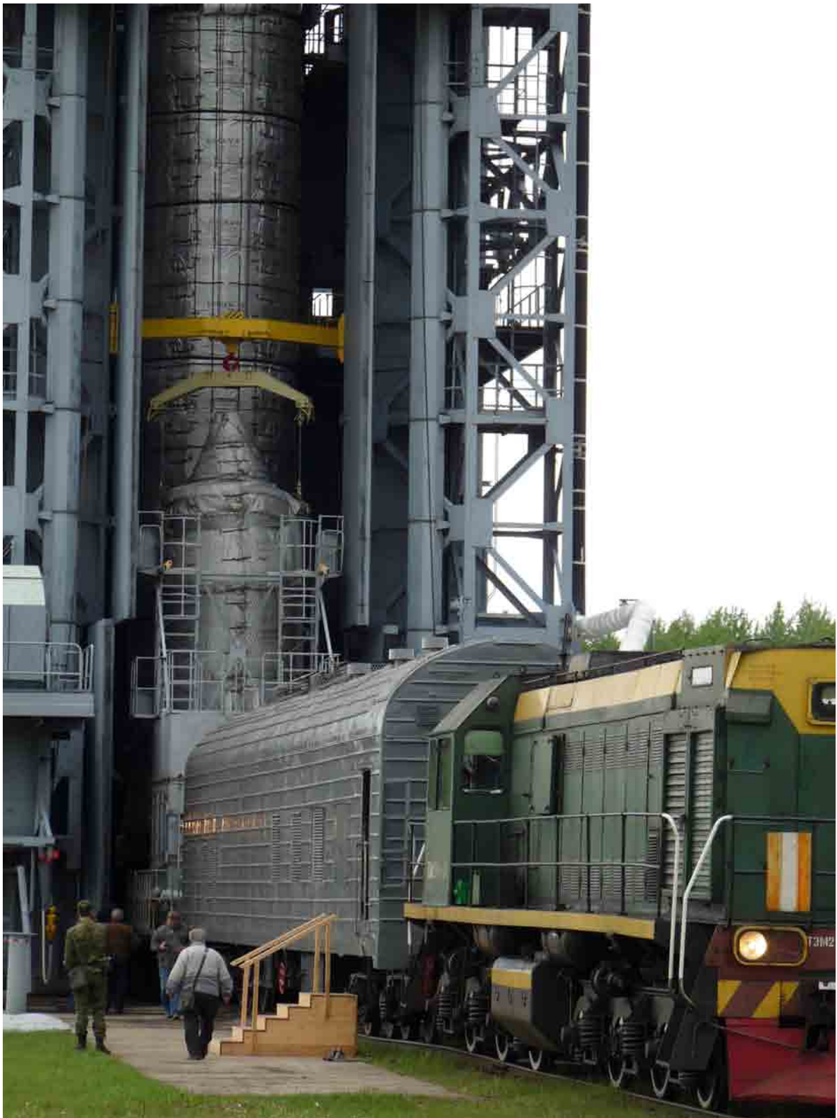
Figure 1-28 Hoisting of upper composite at the Rockot service tower.
