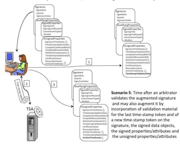
Figure 6: Arbitrator validating a signature with unsigned properties/attributes, requesting a second archive time-stamp token, and augmenting the signature with the validation material and the archive time-stamp token
