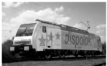
Electric four-system high-performance locomotive ES64F4 for Siemens Dispolok GmbH, Germany
