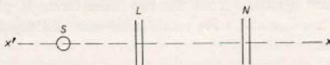
Fig. 6. - Quantal transition of photons issuing from a source S and passing successively two linear polarizers with angles A and B ( \alpha \equiv A - B ).
