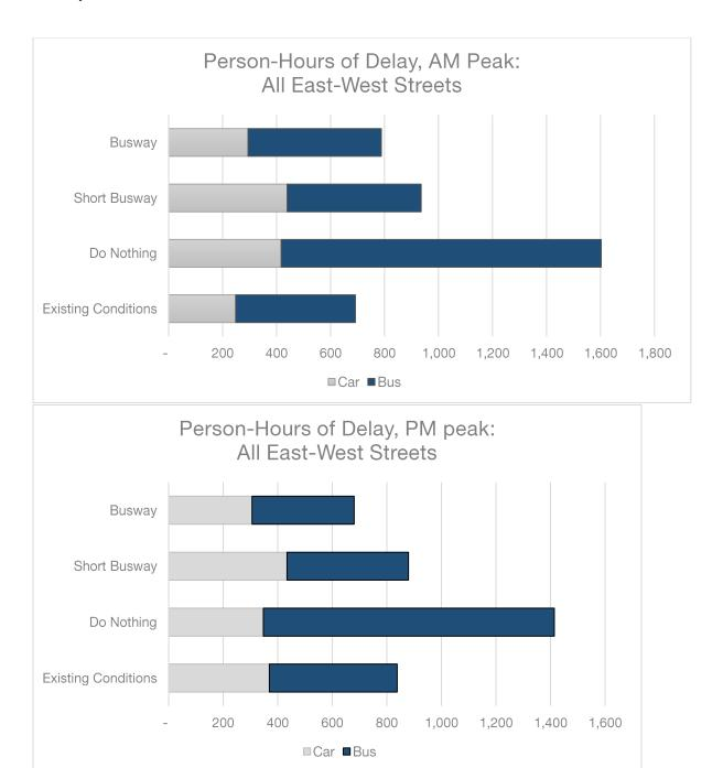
Figure 8: Peak-hour modeled person-hours delay
