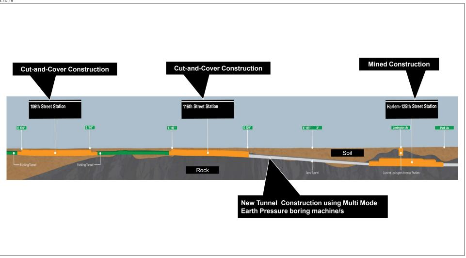
Station, bellmouth structure, and TBM launch site into one continuous structure, and allow for a more compact track design for the bellmouth. As a result, the overall amount of cut-and-cover construction is reduced. These modifications also optimize the TBM construction for the tunnel.
