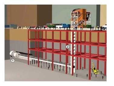
Much of the Second Avenue Subway will be built using tunnel boring technology, in which a powerful circular cutting machine drills a tunnel in rock or soil with minimal disruption to the street  $(\mathbf{1})$ . The excavated material is then taken to street level and removed by truck ((2)). Tunneling will be done through bedrock wherever possible, which is quicker and more cost effective than mining or cut-and-cover.
