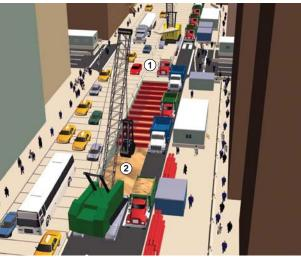
Most of New York City's subway system was built using the cut-and-cover technique. With this method, a trench is cut in the street, the soil is supported by
