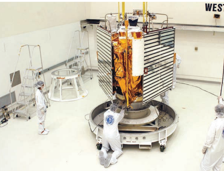
MESSENGER, the first spacecraft dedicated to surveying Mercury, is shown during its construction (left) and depicted in orbit around its target (right).
