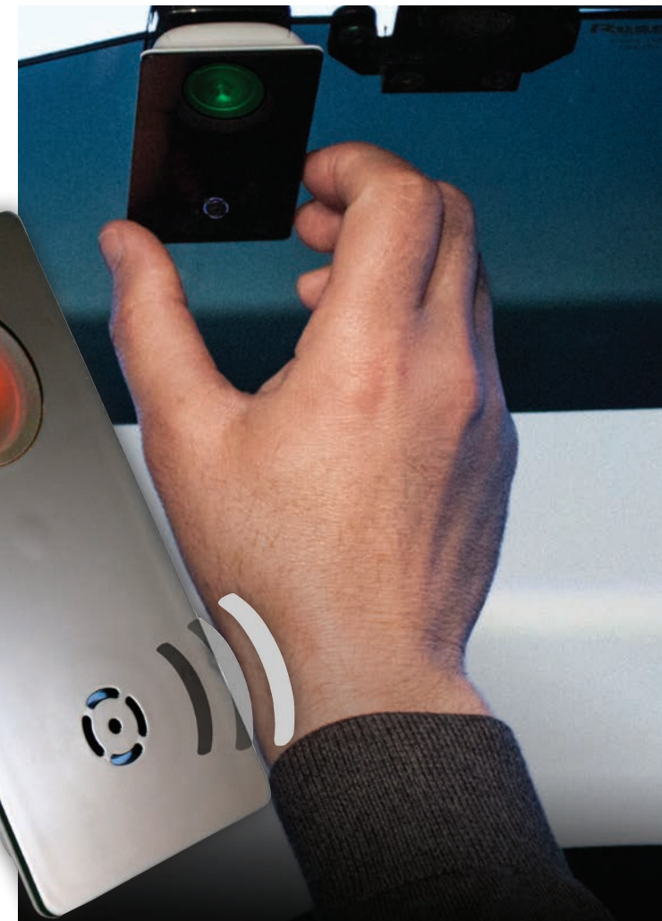
Aviation Technology Inc.'s Alt Alert cabin pressure monitor uses a flashing, red light combined with either advisory chirps or sustained alarms, depending on the seriousness of the situation, to alert pilots and crewmembers to a loss of cabin pressure. The device can be secured to a visor with a clip, but it can also use a suction cup to attach to a window, or Velcro for mounting on an instrument panel.
