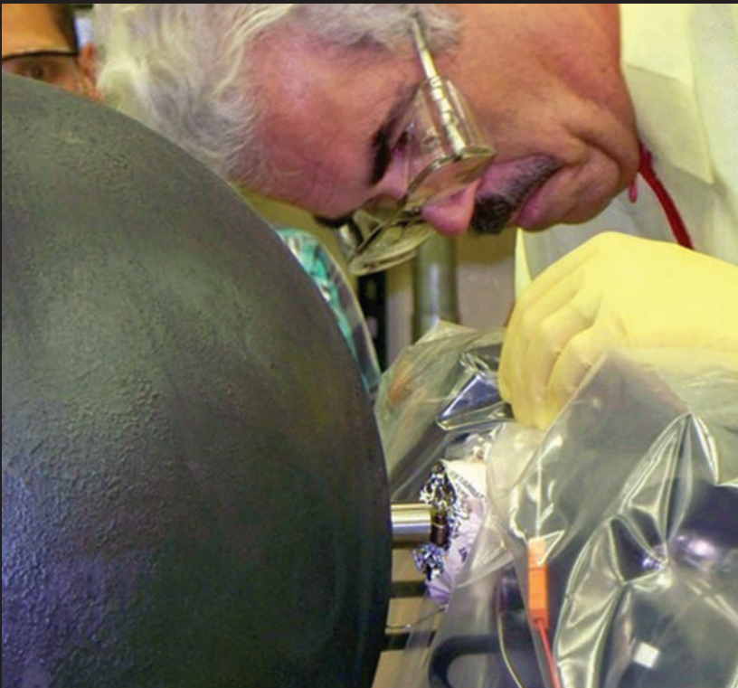
A test operator inserts a water-filled heat pipe into a small nuclear reactor to extract fission heat from the uranium core.
