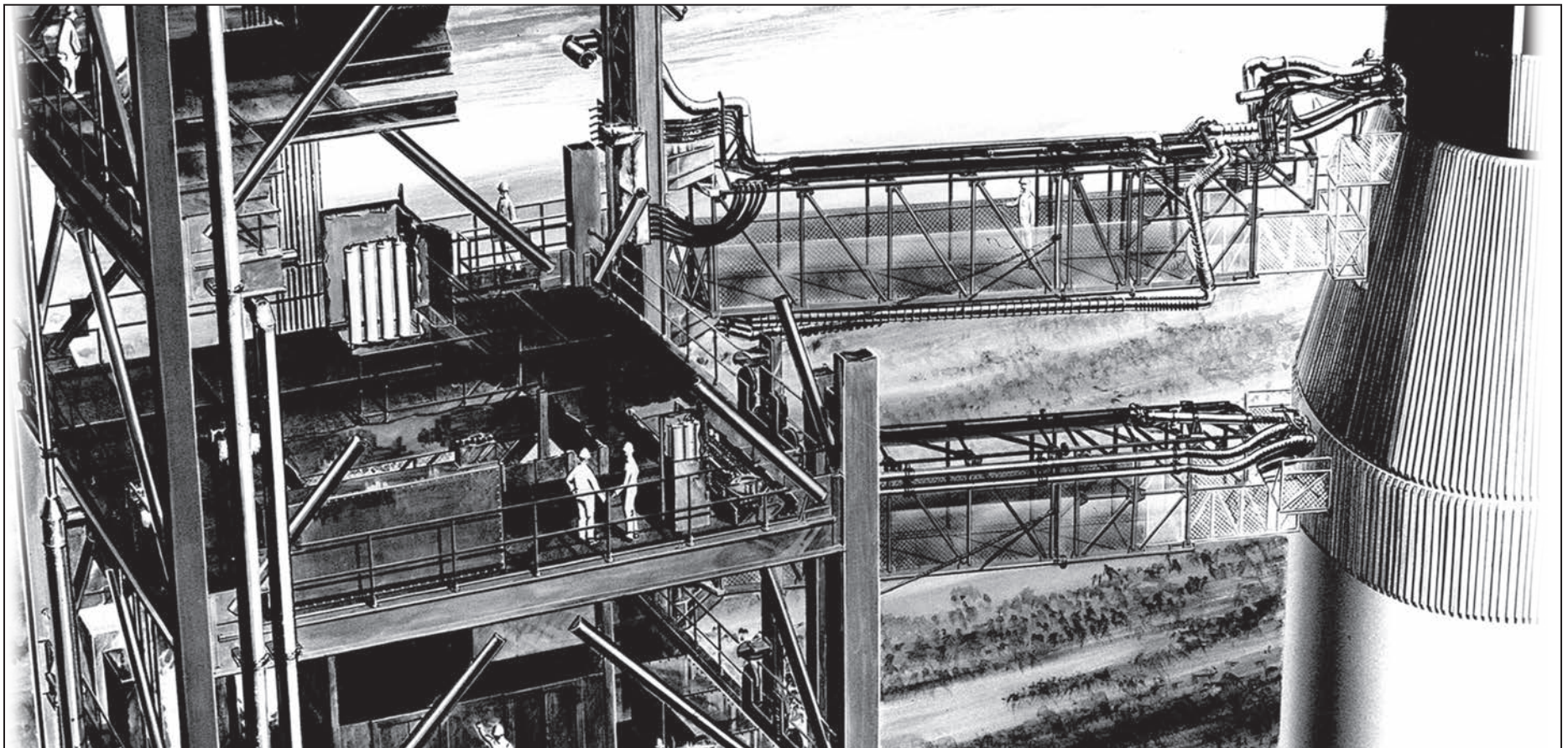
An illustration of the fuel- and electricity-carrying umbilicals that extended from the gantry to the Apollo spacecraft. In the 1960s Taylor Devices developed shock absorbers to help safely dislodge the umbilicals from the spacecraft during launches.
