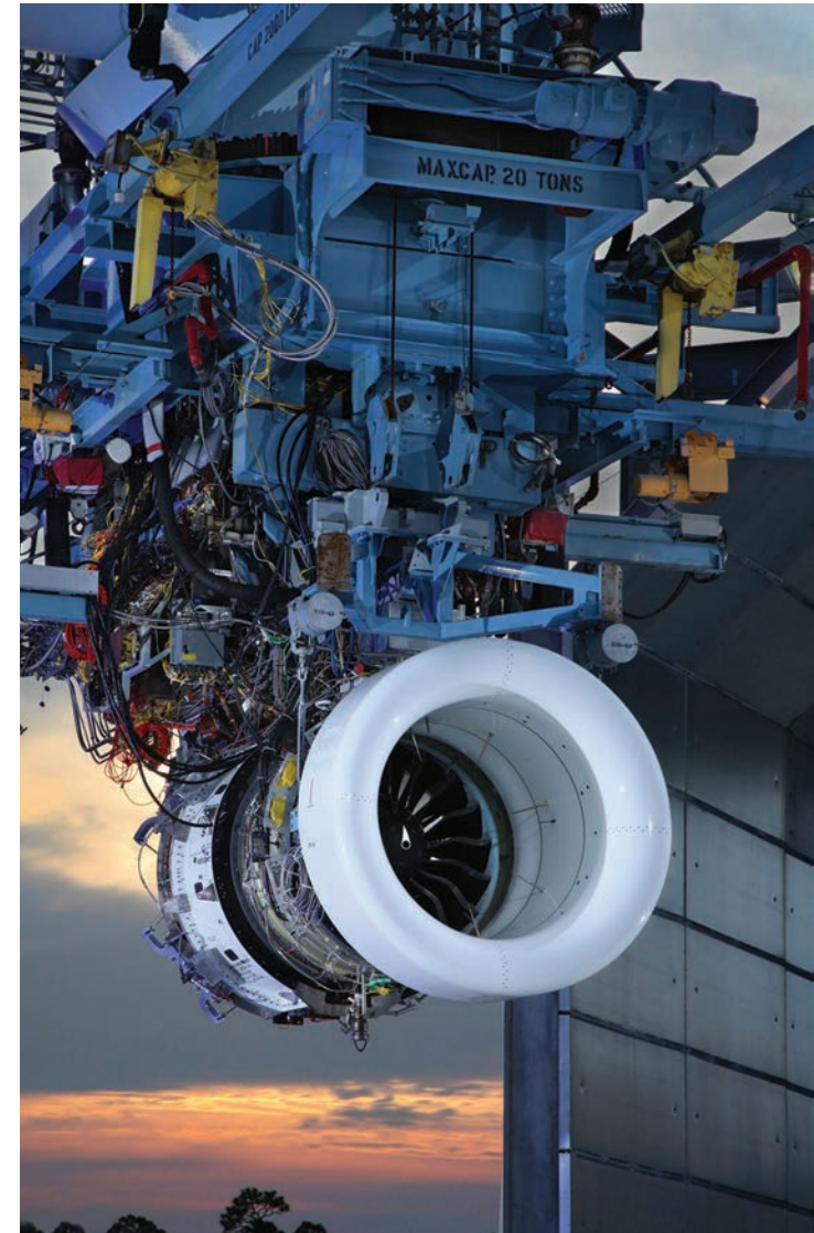
In collaboration with NASA, Pratt & Whitney developed its PurePower family of turbofan engines, which are more fuel-efficient and quieter than other commercial models. Here, the PurePower 1217G engine, developed for Mitsubishi Regional Jet aircraft, undergoes ground testing in West Palm Beach, Florida.
