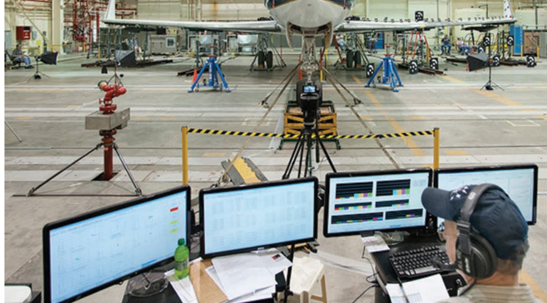
A NASA-invented gas sensor using carbon nanotubes, above left, could find applications in inert gas analysis, thermal conductivity sensing, infrared spectroscopy, and other fields. The Technology Transfer Program just made the patented device available for licensing in 2014. Above right, an Armstrong Flight Research Center flight loads engineer monitors testing of experimental wing flaps that could enable commercial aircraft to be significantly quieter during takeoff, approach, and landing.
