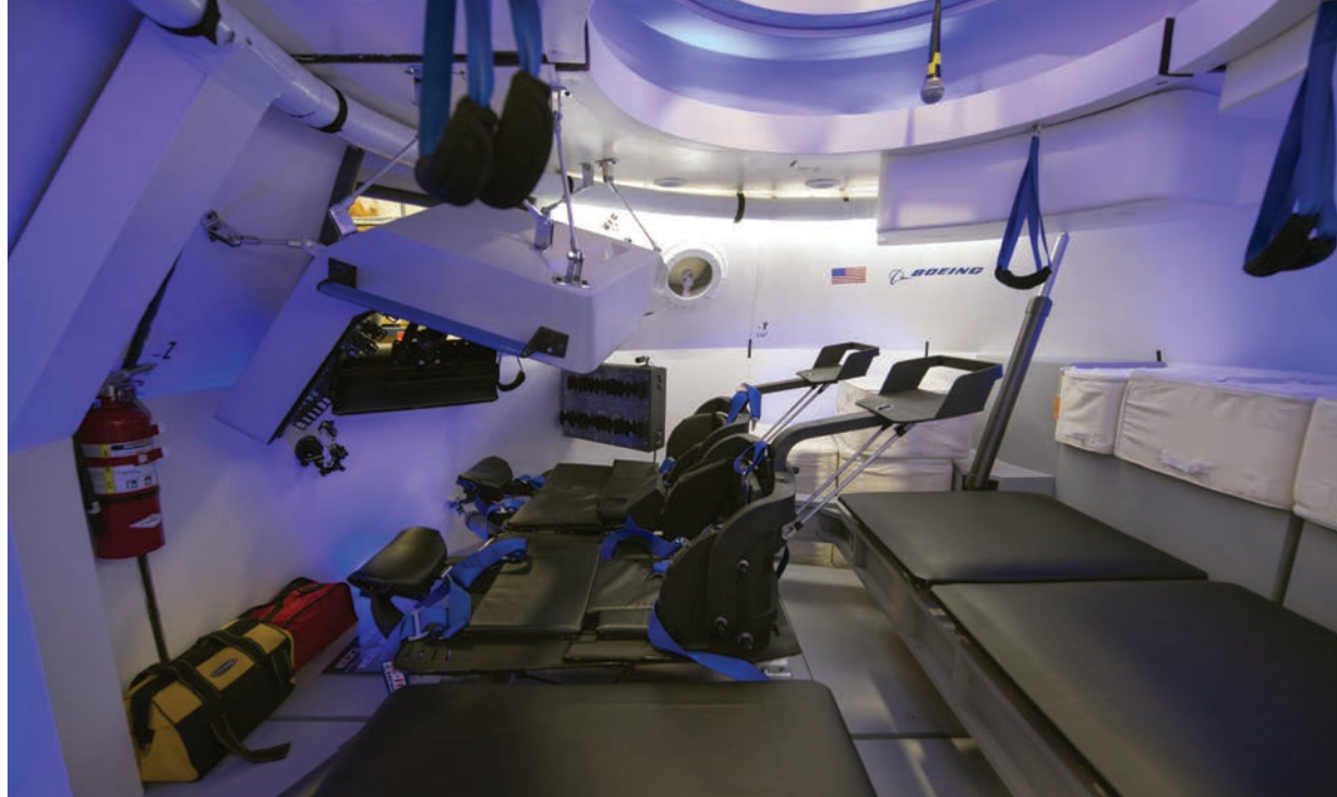
Commercial crew vessels, such as the mockup of Boeing’s CST-100 shown here, are all adopting LED lighting technology as a way to save electricity, extend the life of lighting sources, and potentially help crews manage their biological rhythms as they adjust to life in space.
