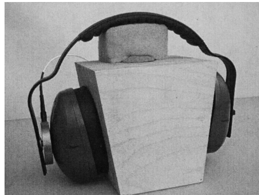
FIG. 10. A photo of the active headset with the PCB actuator mounted between the earshell and the headband.
