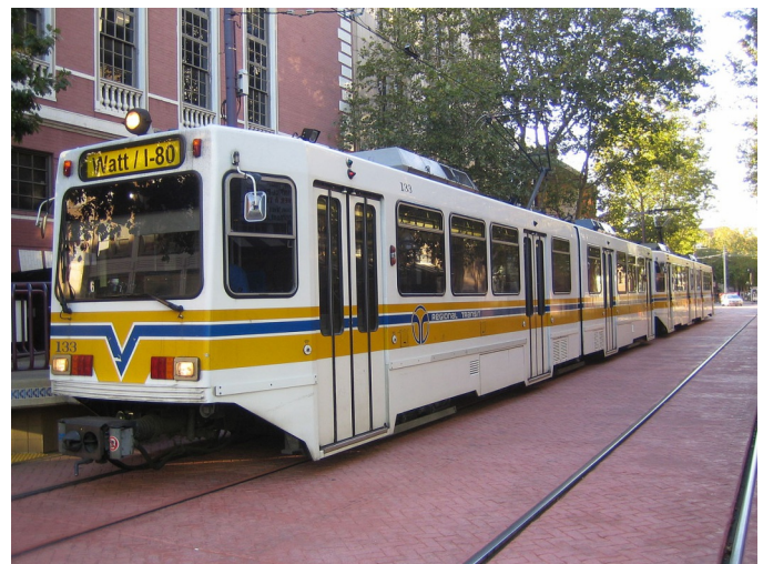
A Siemens Duewag U2A on Sacramento Regional Transit's light rail system in downtown Sacramento. The Siemens-Düwag Type U2A is an upgraded version of the U2 that shares similar characteristics of the newer SD-100s and SD-160s, yet it still uses the mechanical equipment of the U2.
