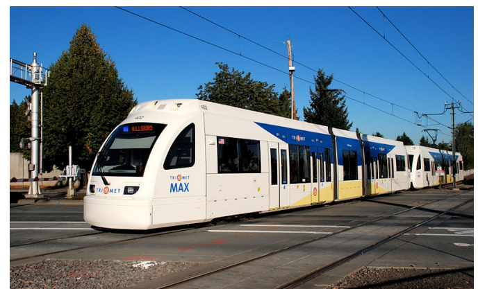
TriMet's Type 4 cars, Siemens S70 LRVs, part of a total order of cars from Siemens of 119 vehicles.
