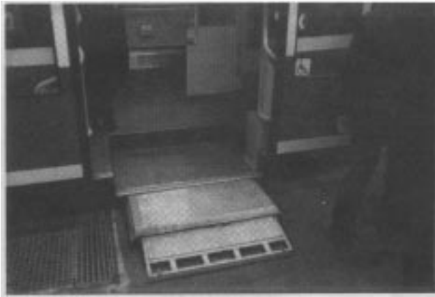
Figure 67. Sliding ramp and lifting bridge used on the AEG (MAN) GT6N LF-LRV in Munich.
