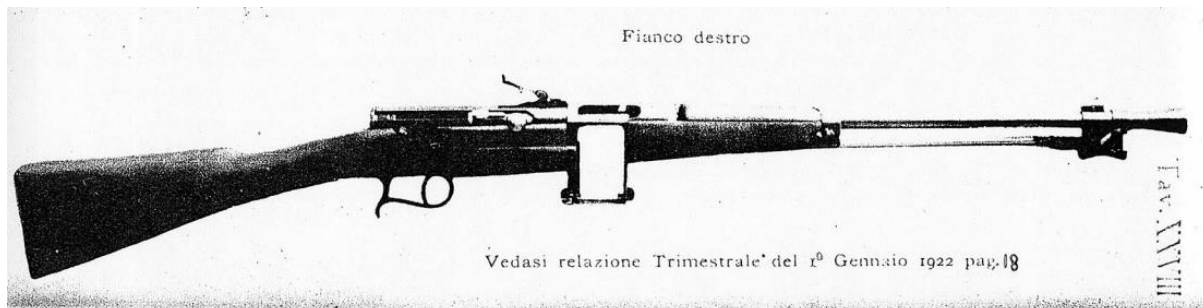
[11.] The Moschetto Automatico Brescia , an intermediate-caliber automatic rifle developed from the Revelli-Beretta in the early 1920s.
