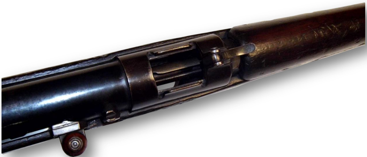
[5.] The cocking slot of the Revelli-Beretta carbine, showing the 45° angled cam slot. This was a carry-over from the Villar Perosa which was intended to create a bolt delay but had little appreciable effect. (Photo: firearms.96.it)
