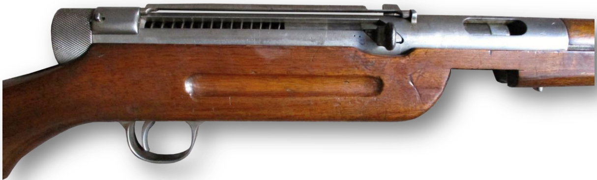
[20.] Detail view of the receiver of the Netsch automatic carbine. It can be seen that this gun uses the same bolt delay as the Villar Perosa and Revelli-Beretta. (Photo: Vojenský Historický Ústav)
