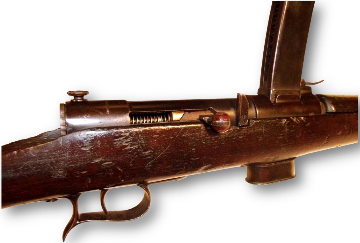
[5.] The cocking slot of the Revelli-Beretta carbine, showing the 45° angled cam slot. This was a carry-over from the Villar Perosa which was intended to create a bolt delay but had little appreciable effect. (Photo: firearms.96.it)
