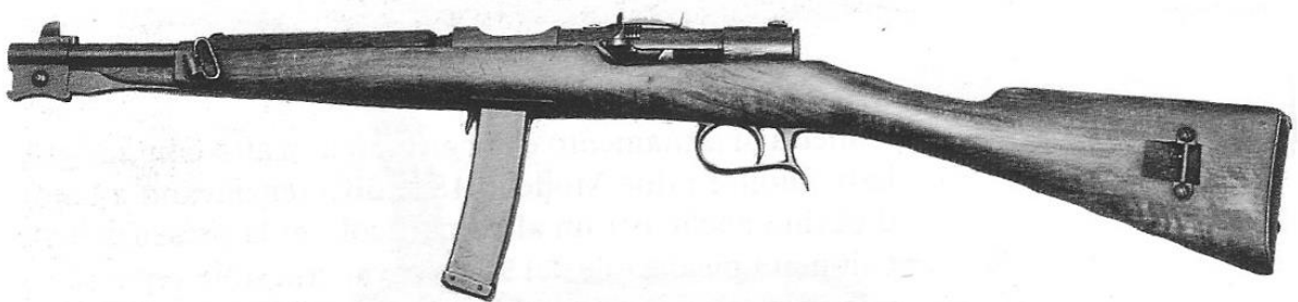
[8.] The inverted-receiver Revelli-Beretta carbine, made on an experimental basis only. The cocking lever is on the left side of the receiver.
