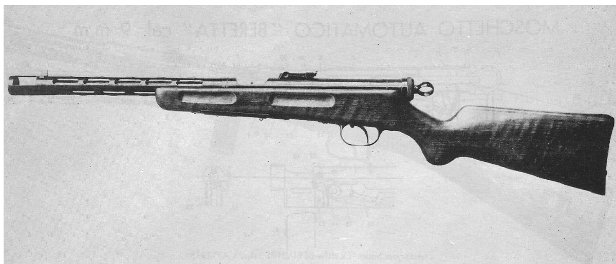
[16.] The Beretta Mod.35, the final iteration in the Revelli-Beretta family and the precursor to the Beretta Mod.38A submachine gun.
