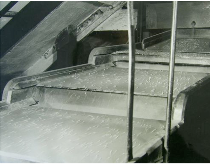
Ap. 15. Shot running on glass. The proper shot had sufficient speed to jump the gaps to the end. However, the imperfect ones fell down and rejected. The picture was probably extracted from the BBC documentary.
