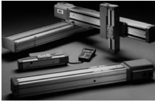
FIGURE 71.11 Cartesian robot. Three-axis robot constructed from modular single-axis motion modules. (Courtesy of Adept Technologies, Inc.)
