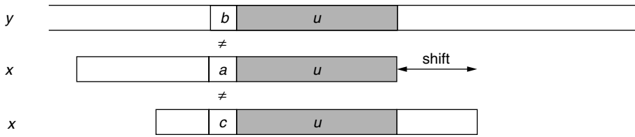
FIGURE 13.7 The good-suffix shift, when u reappears, preceded by a character different from a .
