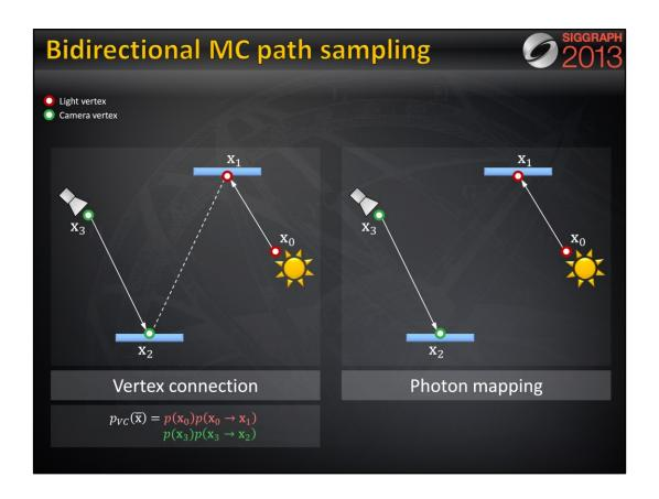
Bidirectional path tracing connects the subpath endpoints deterministically. We call this technique *vertex connection*. The PDF of the resulting full path is well known, and is simply the product of the PDFs of two subpaths, which have been sampled independently.
