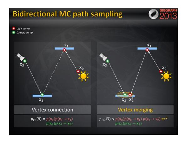
Under the reasonable assumptions that the surface around  $\mathbf{x}_1$  is locally flat, i.e. that this neighborhood is a disk, and that the density of  $\mathbf{x}_2^*$  is constant inside this disc, the integral can be well approximated by the PDF of the actual point  $\mathbf{x}_2^*$  we have sampled, multiplied by the disc area  $\pi r^2$ .
