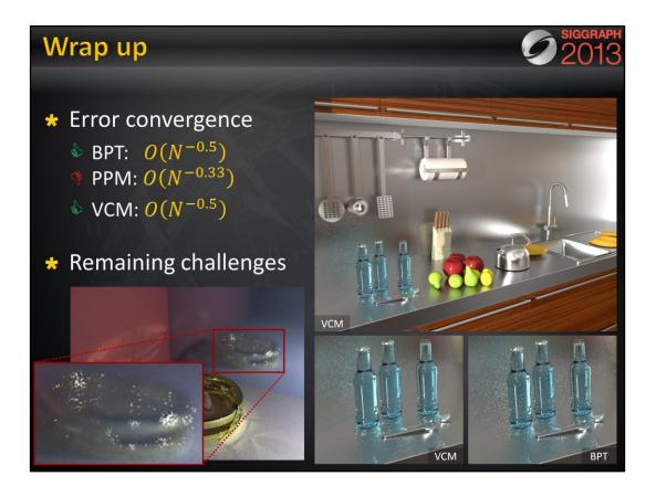
In summary, vertex connection and merging tries to combine the best of bidirectional path tracing (BPT) and (progressive) photon mapping. An important property of the algorithm is that it retains the higher order of convergence of BPT, meaning that it approaches the correct solution faster than PPM as we spend more computational effort (i.e. sample more paths). The asymptotic analysis can be found in the VCM paper.
