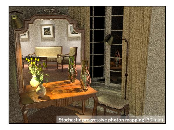
On the other hand, photon mapping (PM) is well known for its efficient handling of caustics. Recently, Hachisuka and Jensen [2009] showed a progressive variant of PM that converges to the correct result with a fixed memory footprint. Their stochastic progressive photon mapping (PPM) algorithm captures the reflected caustics in our scene quite well. However, it has hard time handling the strong distant indirect illumination coming from the part of the scene behind the camera.
