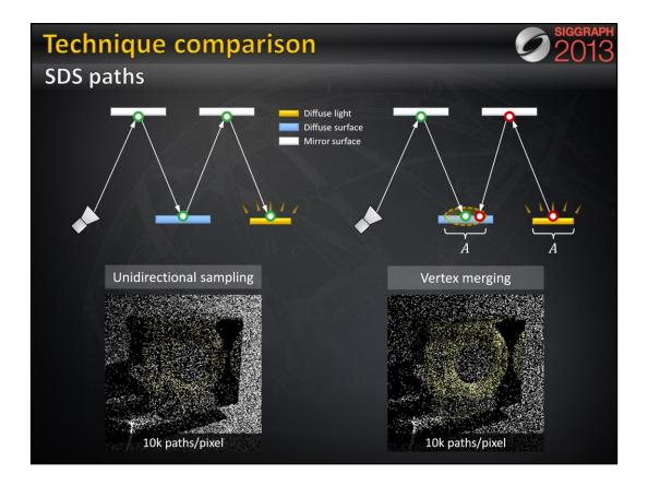
To answer this question, let us first take a look at specular-diffuse-specular (SDS) paths. Here, bidirectional path tracing can only rely on unidirectional sampling: it traces a path from the camera hoping to randomly hit the light source. With vertex merging, we can trace one light and one camera subpath, and merge their endpoints on the diffuse surface.
