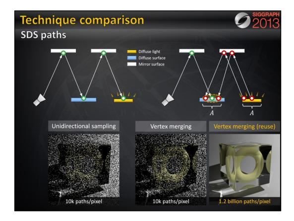
However, the strength of vertex merging is computational efficiency – we can very efficiently reuse the light subpaths traced for *all* pixels at the cost of a single range search query. This allows us to quickly construct orders of magnitude more light transport estimators from the same sampling data, with a minimal computational overhead, resulting in a substantial quality improvement.
