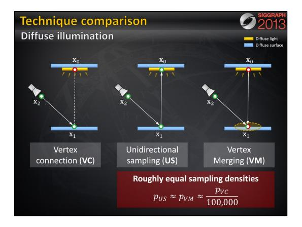
Now let's look at another extreme example – diffuse illumination. Note that vertex connection (VC) constructs the edge between  $x_1$  and  $x_2$  deterministically, while unidirectional sampling (US) and vertex merging (VM) both rely on random sampling.
