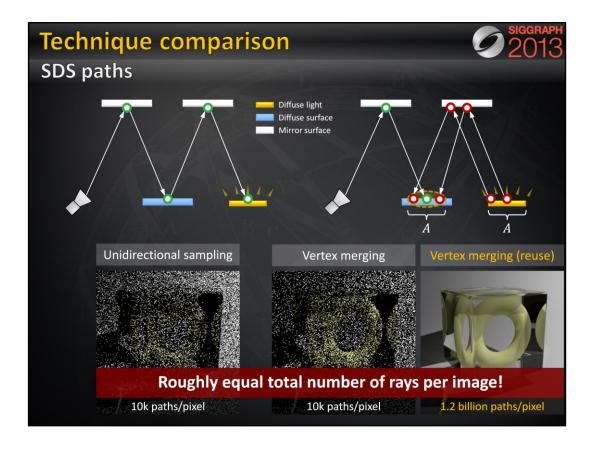
For all these three images we have traced roughly the same number of rays, and the only difference between the one in the center and the one on the right is that the for right image we have enabled path reuse, by storing, and looking up, the light subpath vertices in a photon map at every rendering iteration.
