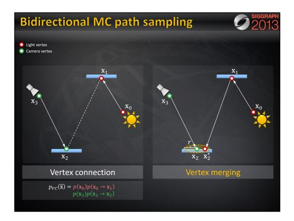
We label this technique *vertex merging*, as it can be intuitively thought to weld the endpoints of the two subpaths if they lie close to each other.
