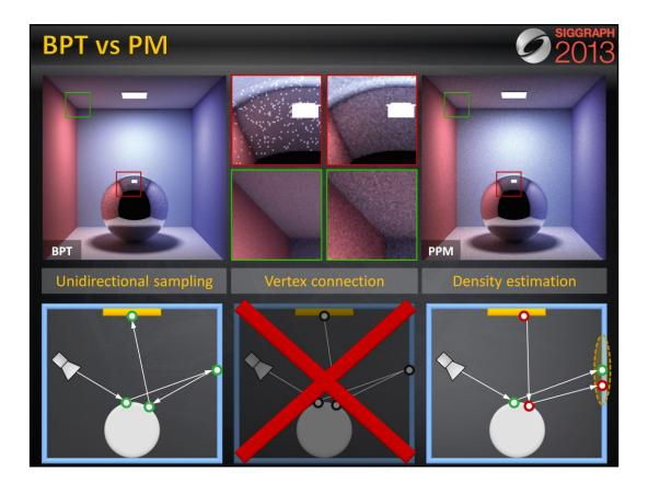
BPT can efficiently capture directly visible caustics, as it can connect light subpath vertices to the camera. However, for sampling specular-diffuse-specular paths, BPT can only rely on unidirectional sampling, as VC cannot perform connections with specular vertices. Since the probability of randomly hitting the light source is often very low, the resulting images suffer from excessive noise.
