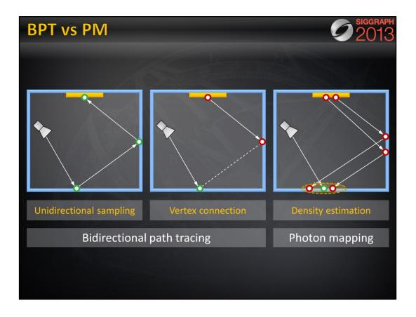
Let us start by reviewing how bidirectional path tracing (BPT) and photon mapping (PM) sample light transport paths that connect the light sources to the camera:
