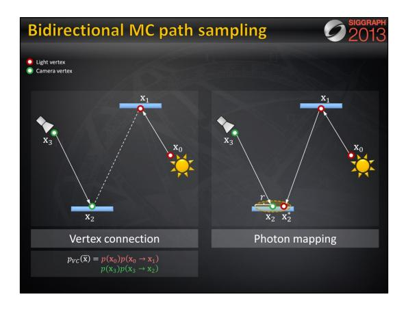
Photon mapping, on the other hand, will extend the light subpath by sampling one more vertex from  $\mathbf{x}_1$ , and will concatenate the two subpaths only if the "photon" hit-point  $\mathbf{x}_2^*$  lies within a distance r from  $\mathbf{x}_2$ .
