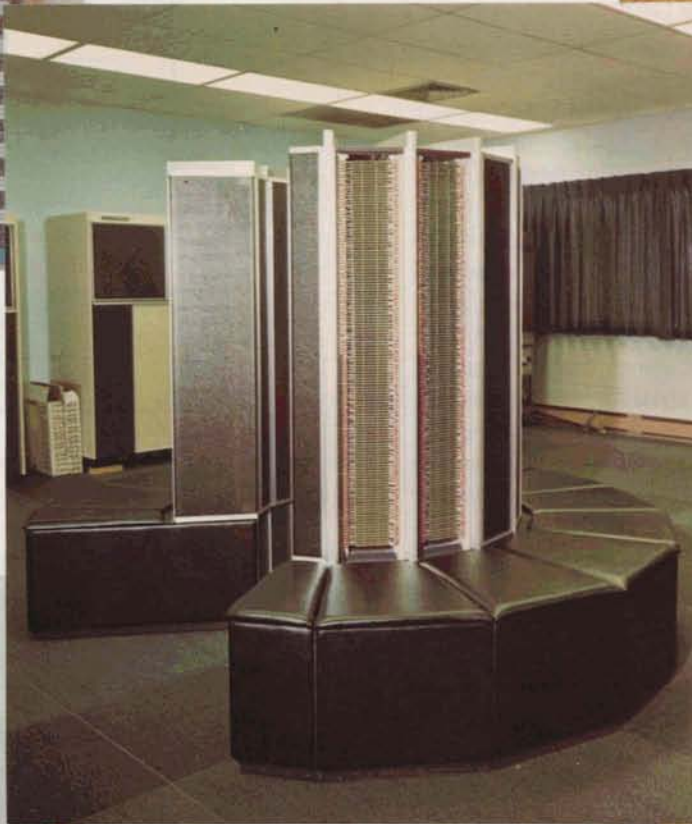
CRAY-1 computer shown with installed banks of printed circuit board modules.
