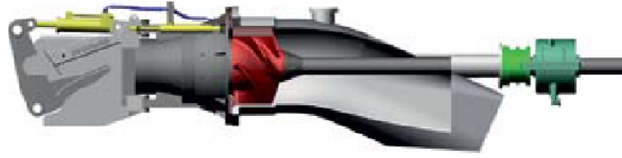
Figure 6.3: X-ray view of a water jet, produced by Wartsilla [58].
