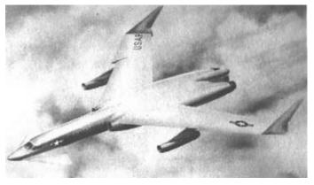
This strange experimental aircraft, the Convair NX-2 was to be built (two of them) to test the General Electric and Pratt & Whitney nuclear engines. Effectively, an atomic version of the J-58 was seriously considered. © Convair
