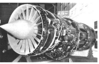
The SNECMA Company considered building the M35, which was the equivalent of the JT11B built under license for the supersonic transport airplane project (future Concorde). It is without doubts the reason that Pratt & Whitney introduced this J-58-P2 at the 1963 Le Bourget air show, whereas the "Blackbird" the only airplane equipped with this engine was still totally unknown. Its existence was indeed not revealed until February 29, 1964.
