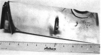
First stage turbine blade of the same J-58 after impact by a flashlight.  $\ensuremath{^\odot}$  Lockheed
