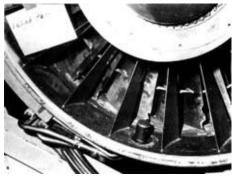
J-58 air inlet after the ingestion of an inspector's flashlight in charge of checking for foreign objects...Total damages: \$ 250,000. © Lockheed
