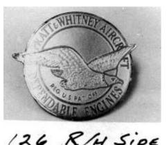
J-58 metal insignia almost intact after being ingested by its compressor. After that, the factory marking was engraved directly on the engine case. © Lockheed
