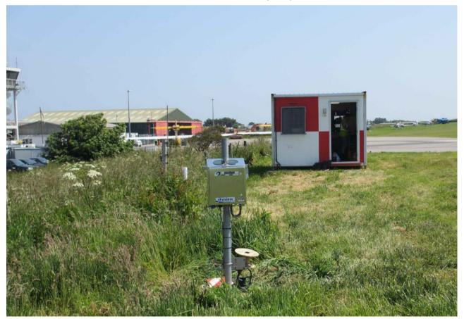
The new Alderney Airport laser ceilometer is installed - the instrument is capable of measuring cloud base heights up to 24,000 feet above the airfield.
