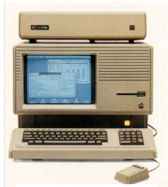
Apple Lisa with a ProFile hard disk on top
