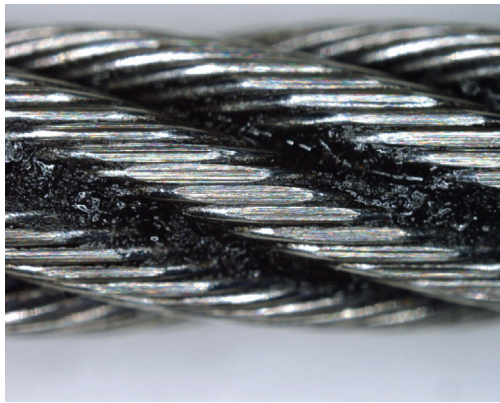
Binocular view of the wear area on a stainless steel cable after 150,000 cycles
