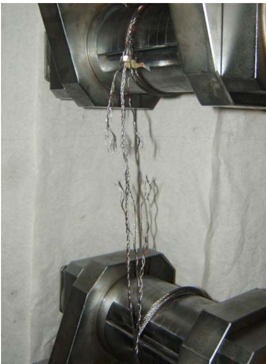
View of pitch-down cable on traction machine : high degree of untwisting
