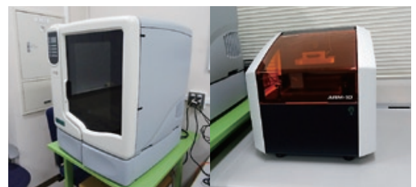
▲ 3Dプリンタ（熱溶解積層式と光造形式） 3D Printer (by Fused Deposition Modeling and Optical Stereolithographic Method)
