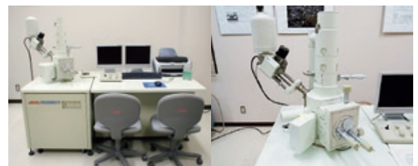
▲ 走査型電子顕微鏡・X線分析装置 Scanning Electron Microscope and Energy Dispersive Spectrometer
