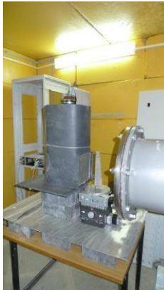
Neutron imaging instrument: Sample and detector position
