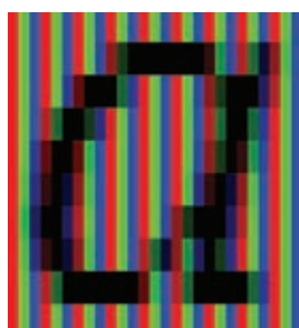
ClearType rendering using individual subpixels results in smoother curves and more natural diagonal strokes.
