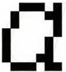
An italic letter hinted for black & white display. The outline is distorted by hint instructions to turn on or off specific pixels.
