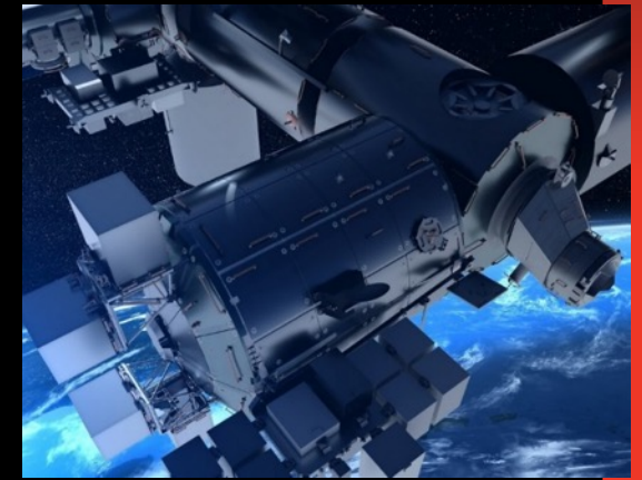
Bartolomeo payload platform on Columbus Module holds up to 11 external units (image credit: ESA)
