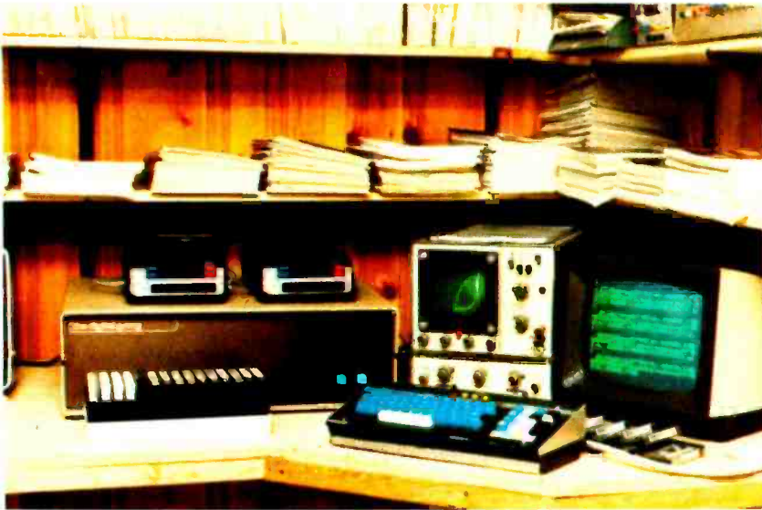
Photo 1: The author's computer system, showing the address state analyzer in operation with a BASIC program (see oscilloscope in center of picture). The program is printing an integer sequence of ASCII characters on the display to the right using the function CHR$(X). On the left is a 50 K byte Digital Group Z-80 system.
