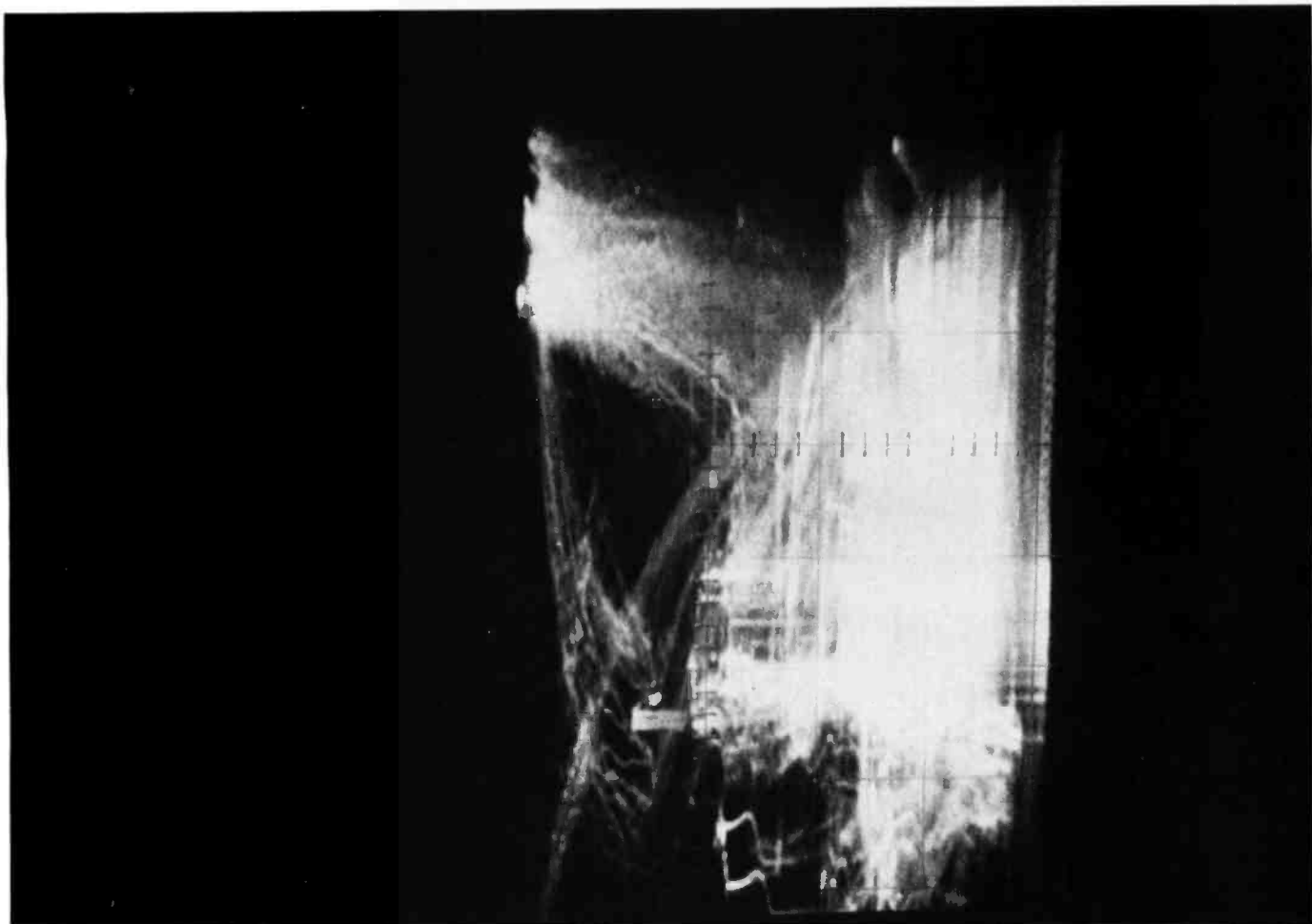
Photo 4: A complex bus addressing pattern during the execution of a BASIC program.
