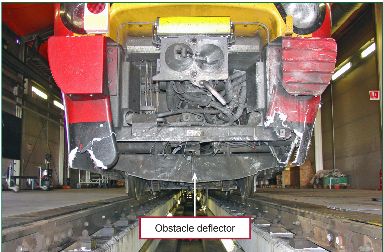
Figure 8: Obstacle deflector at the front of the train after the accident
