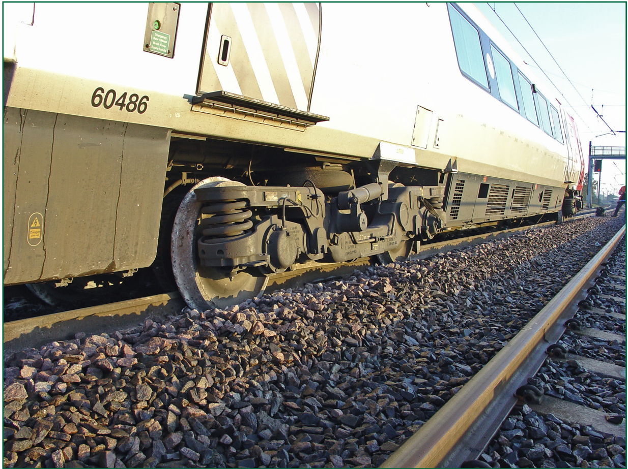
Figure 4: The derailed wheelsets, 2, 3 and 4 from the front, on the leading vehicle
