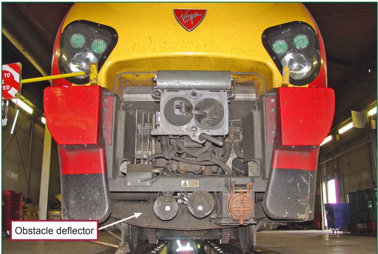
Figure 7: Undamaged obstacle deflector at the rear of the train (note that horn covers are missing)
