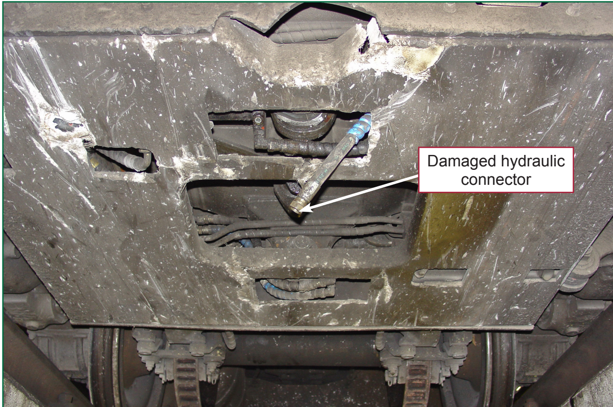
Figure 10: Stone guard showing openings and damaged hydraulic connector
