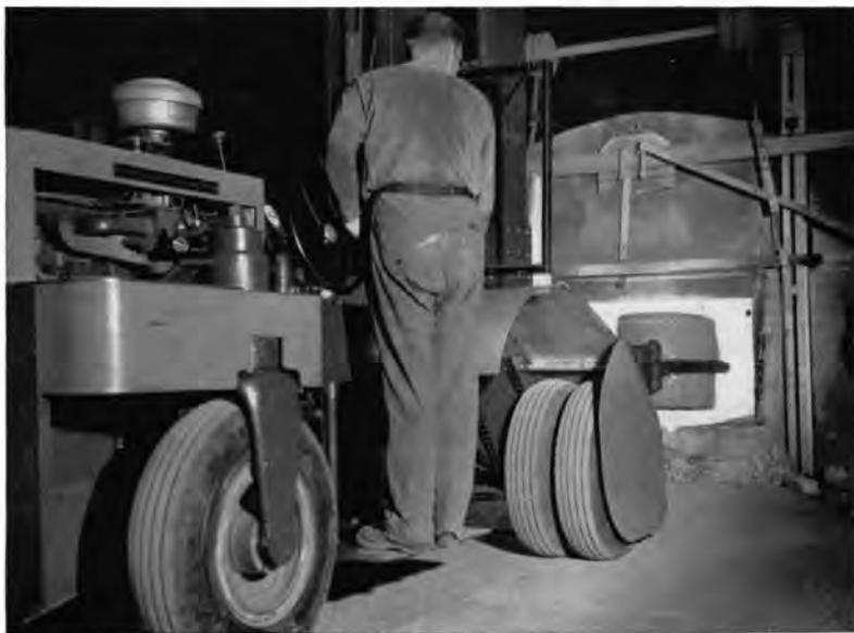
The pot of glass is placed in and removed from the furnace by means of this specially designed ten-ton truck.
