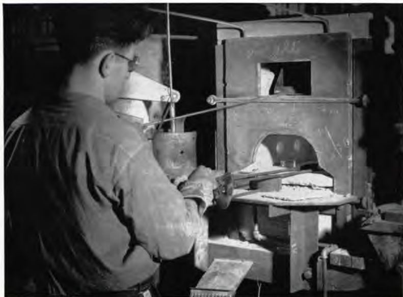
At these furnaces the glass squares are molded into rough lens blanks, preparatory to grinding and polishing.
