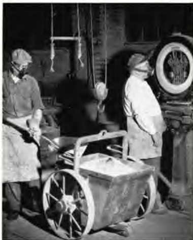
The raw materials for making glass are accurately weighed out according to definite formulas.
