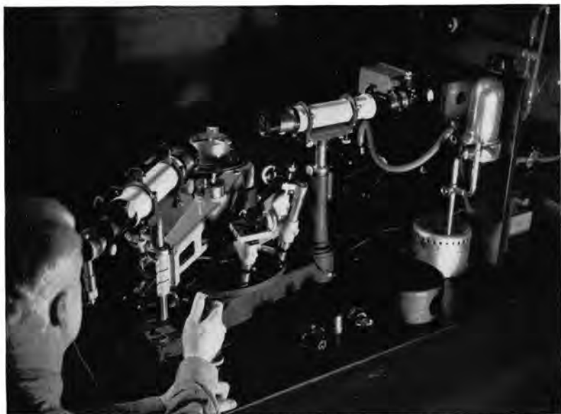
The Spectrometer is used by B&L scientists for ultra-precise refractive index measurements, which are essential in optical science.
