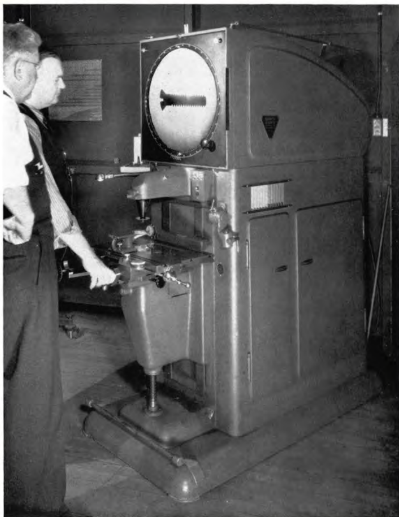
The Contour Measuring Projector is used to examine and measure small machine parts and products, more precisely and speedily than by any other method.
