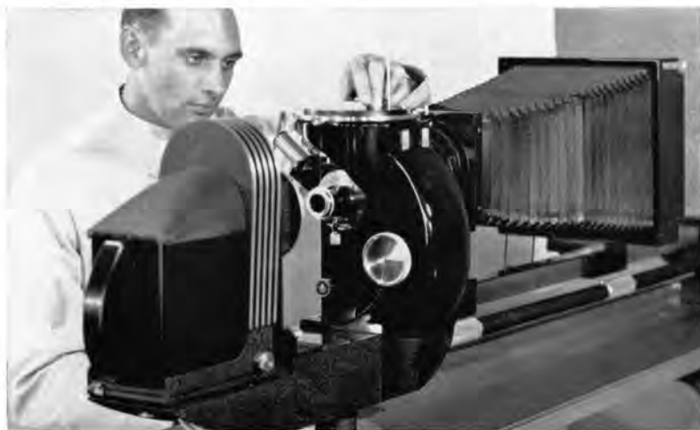
The Research Metallographic Equipment is used extensively in industries the world over for visual observation and photography of metals.
