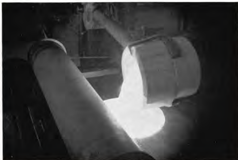
The truck transports the pot of molten glass to the casting table, where the glass is poured and rolled into a sheet of desired thickness.
