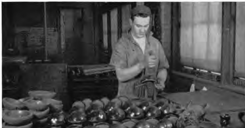
Preparatory to grinding and polishing, the rough lens blanks are attached to grinding blocks by means of pitch and rosin.
