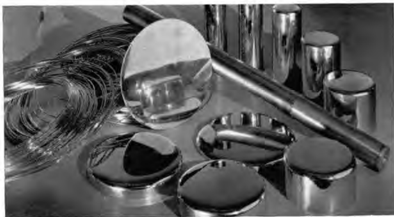
In making gold filled eyewear stock, a cylinder of gold is soldered to a rod of optical metal, then drawn through diamond points into wire stock.
