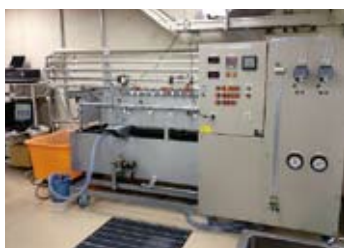
◀ 管摩擦実験装置 Pipe-friction experimental device
