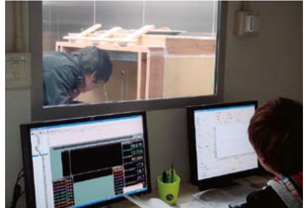
▲ 計測実験の様子：人工気候室での温熱環境実験 Measurements and experiments of the thermal environment
