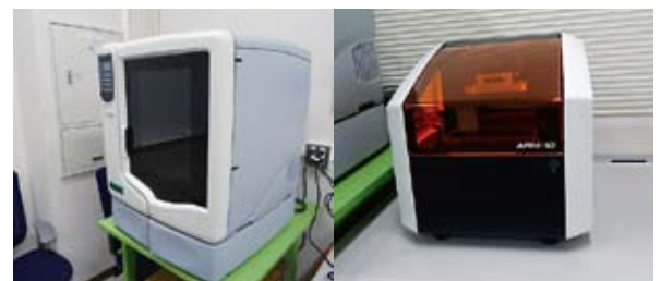
▲ 3Dプリンタ（熱溶解積層式と光造形式） 3D Printer (by Fused Deposition Modeling and Optical Stereolithographic Method)
