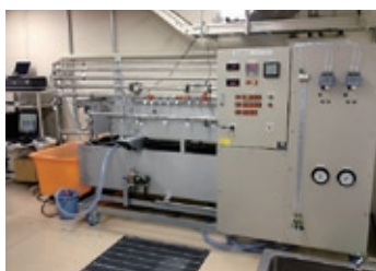
◀ 管摩擦実験装置 Pipe-friction experimental device
