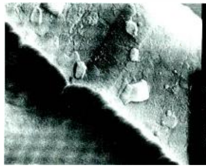
Fig. 1b—6000X magnification shows excellent metal coverage over an oxide step.
