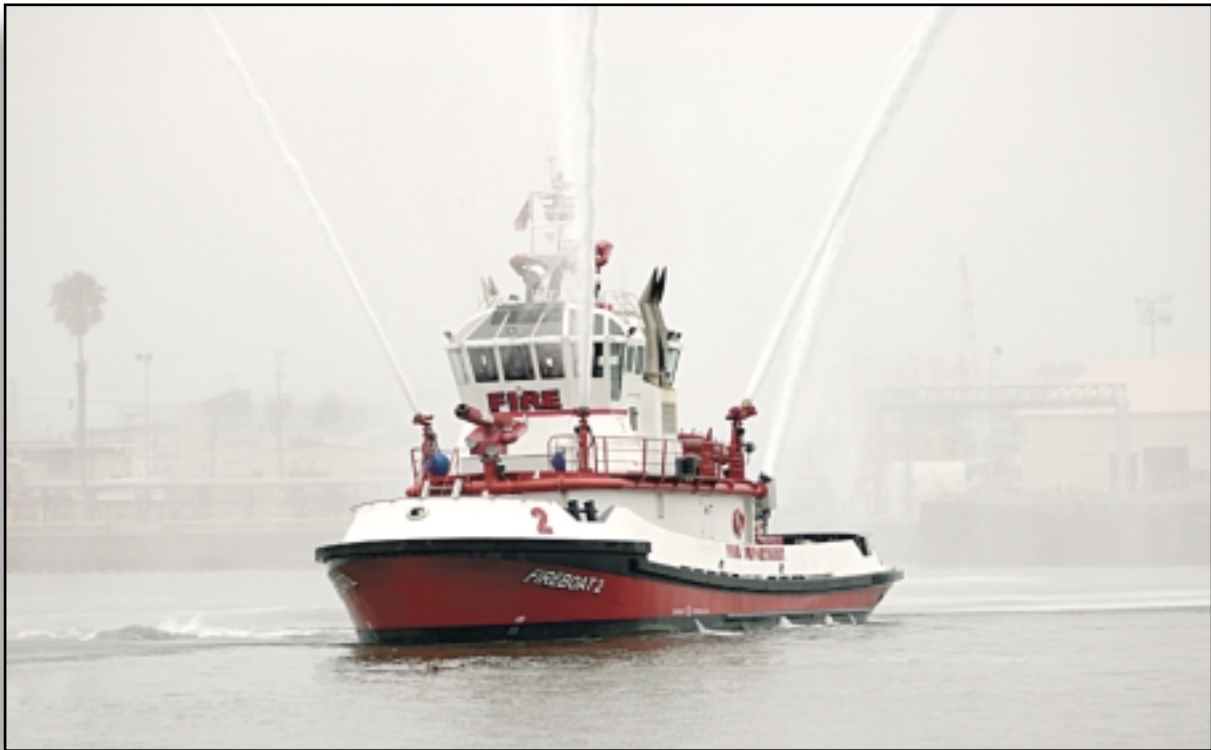
Figure 3.41 – Modern Tug with Fire -fighting Capabilities
