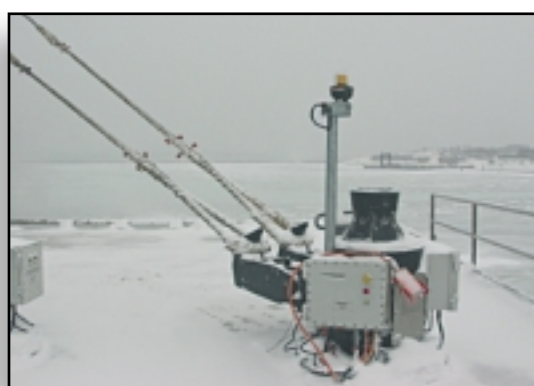
Figure 3.9 – Vertical Angle Mooring Line Reproduced with permission from Harbour & Marine Engineering www.harbourmarine.com
