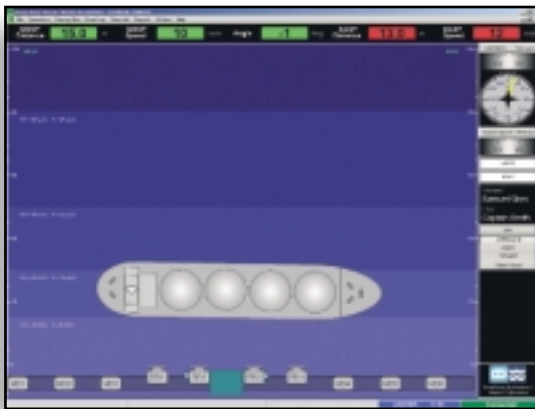
Figure 3.35 – SmartDock® DAS Screen for an LNG Vessel
