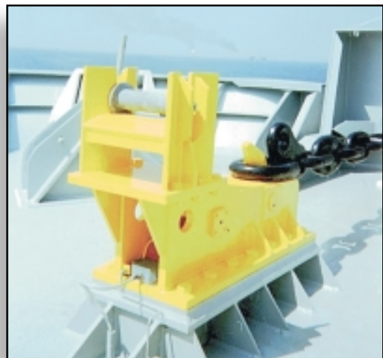
Figure 3.22 – Quick-release Chain Hawser Hook Fitted with Hydraulic Remote-Release, Load Pin and Hawser Fast Lead
