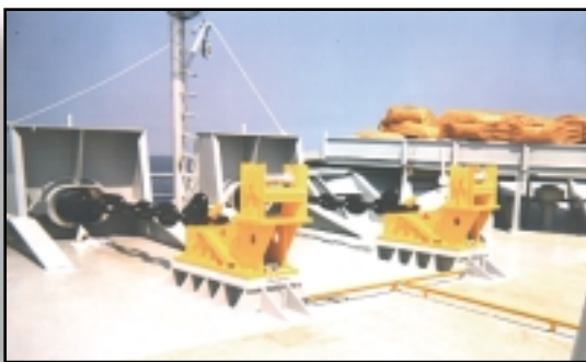
Figure 3.21 – Bow-mounted Twin Hawser Hooks on Texaco's FSO 'Lombo Este', Angola
