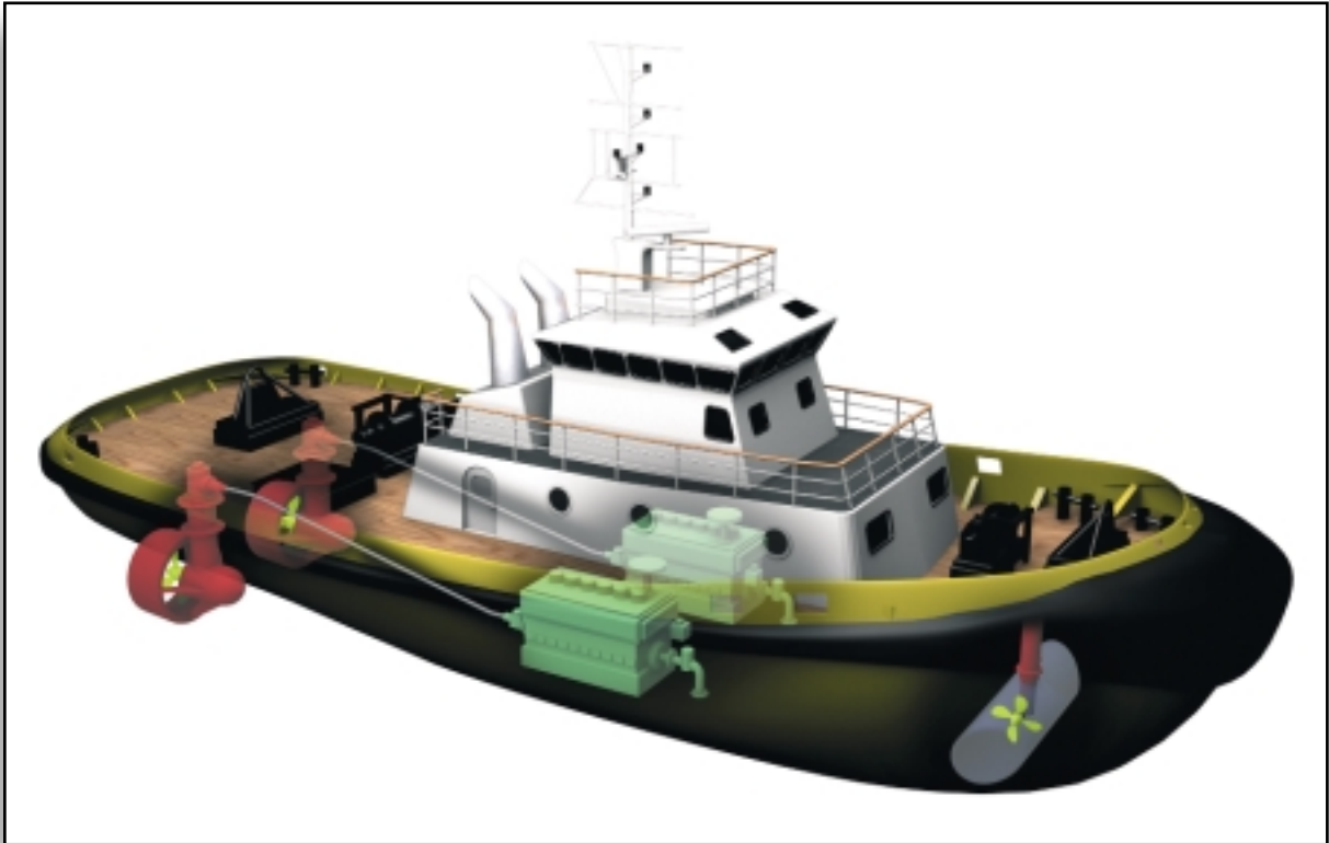
Figure 3.45 – Azimuth Stern Drive Tug
