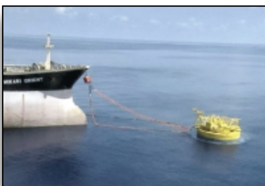
Figure 3.16 – Single Point Mooring System Reproduced with permission from Harbour & Marine Engineering www.harbourmarine.com
