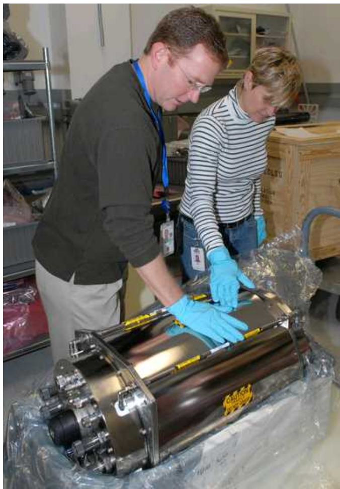
図4.1-4 STS-119で運ばれた交換用のDistillation Assembly (DA) (NASA KSC) http://mediaarchive.ksc.nasa.gov/detail.cfm?mediaid=39583
