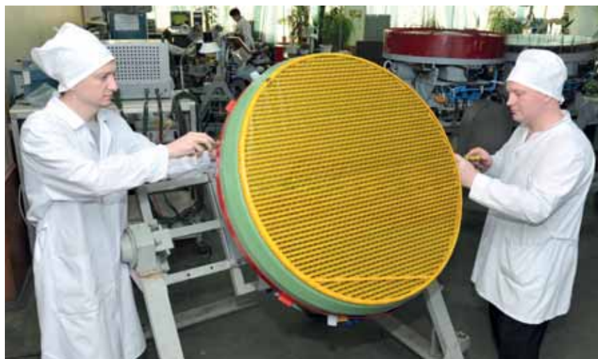
Assembly of an Irbis fire control radar phased array antenna
