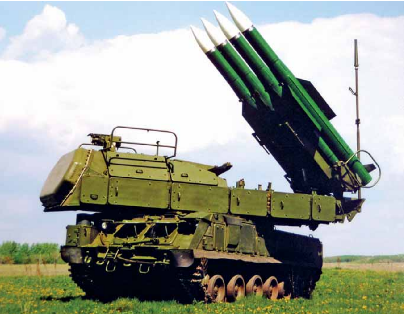
Fig. 6. Multifunction radar on the self-propelled tracked chassis
