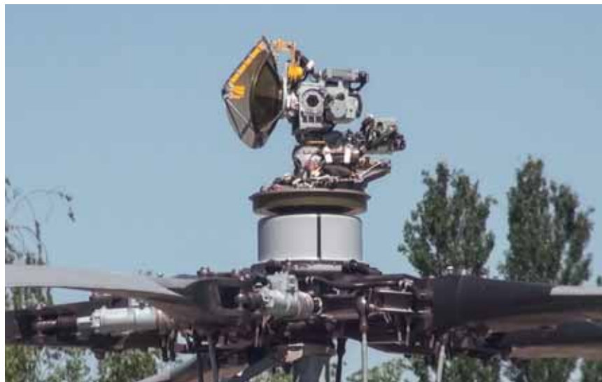
A GRPZ-developed radar onboard a Mi-28N helicopter
